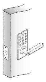
At the heart of the system is an electric motor controlled by electronic circuitry to transition the lock to or from a locked or unlocked state. Electric motor failure is 'critically bad.'
