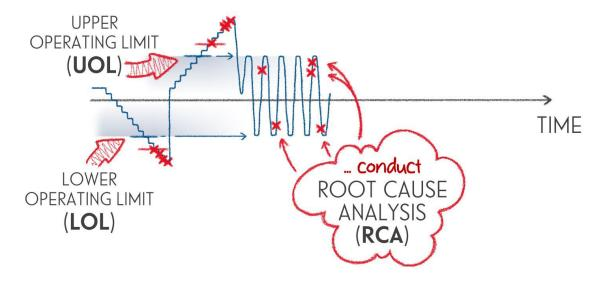
The reason we want to do this rapid cycling of temperatures is that it will force the PCB and its components to grow and shrink based on their coefficients of thermal expansion. Different component will expand and shrink at different rates. This introduces stresses and strains that mimic many of the fatigue and shock stresses the PCB will experience during its normal life. And this is how HALT will induce failure.
