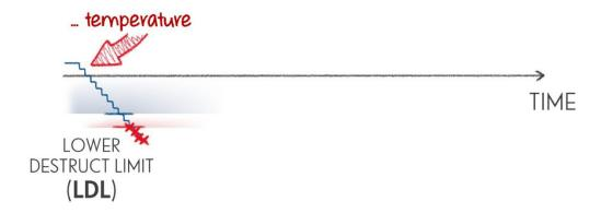
We would obviously see several more failures before we decide to stop that part of the test. The next part of the test is the 'hot thermal stress step test' where we essentially repeat the first part of the test, but with increasing temperature.
