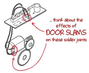
Perhaps qualification testing will uncover this critical design flaw ... as our lock needs to be able to withstand multiple shock forces when the door it is installed on is slammed (which a significant number of our future customers will no doubt do.) Unsecured cables in our smart lock that are only physically restrained with solder is a recipe for failure.
