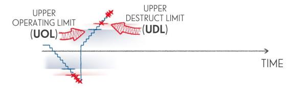
We then get two more higher temperatures that define the Upper Operating Limit (UOL) and the Upper Destruct Limit (UDL). But now we need to do something different. Instead of pushing temperature too far in either direction, we now oscillate temperatures between the UOL and LOL. This will typically induce failures that we then subject to more RCA to come up with more CAs.
