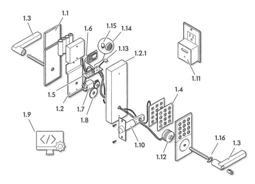
When we design something that is 'novel' or 'cool' we can often overlook the simplest of things. Like electric cables that connect the electric motor to the Printable Circuit Board (PCB). A **BUILD-TEST-FIX** approach means building a prototype that uses soldered cable that is not resilient to shock loads that are generated when a user or customer slams the door shut.
