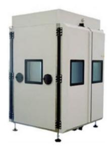
The chamber contains a table upon which systems and components can be secured and then subjected to random vibrations (with six degrees of freedom) up to 75 g RMS. It can also rapidly cycle temperature between 200°C to -100°C. The temperature cycling simulates cycling stresses as adjacent components have different coefficients of thermal expansion.
