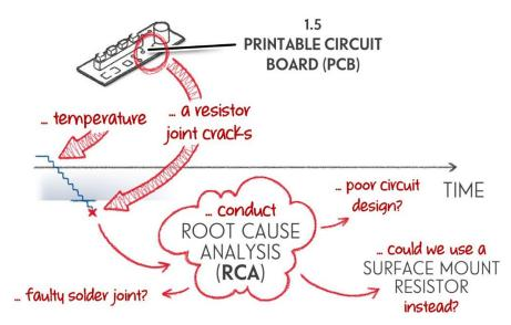
We can then 'patch up' the PCB and keep testing. The cold temperature at which we experience that first failure is the Lower Destruct Limit (LDL).
