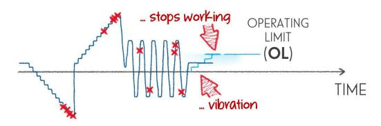
We keep increasing the vibration until the capacitor breaks free. This is the Destruct Limit (DL) for vibration.
