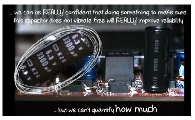
The system is then repaired, and testing continues until a prioritized list of likely failure mechanisms emerges. Or ... the **VITAL FEW**. **HALT** involves increasing well known stresses in a controlled, but not scientific way. We keep increasing the stress to identify WHAT will break. This can help us then understand HOW our product will fail. **HALT** can't measure, it can only point us in the right direction.
