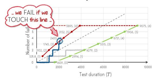
This new demonstration test plan now allows 'early termination' if the product doesn't perform well early. This saves time and money (including in terms of the number of prototypes or units under test).
