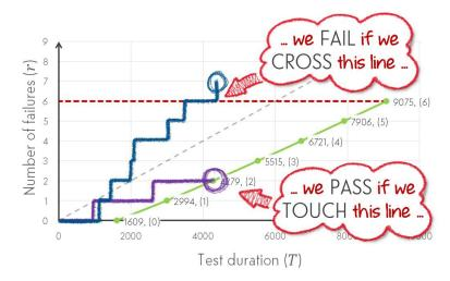
This test plan ensures that if any product 'passes' the test, it will meet the MTBF requirements (1 000 km with 80 % confidence) outlined previously. It also ensures that a product with an actual MTBF of 2 000 km (Discrimination Ratio of 2.0) will have an 80 % probability of passing.
