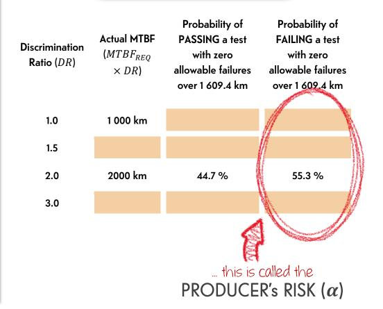
So if the **producer's risk** ( $\alpha$ ) is too high, we increase the number of allowable failures and repeat the process. This gives us the following values
