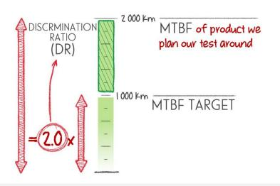
Now we need to use our **Poisson distribution** to understand the probability of our 'more reliable' failing any test in order to quantify the **Producer's Risk**. And the reason we can do this is because we are assuming a constant **hazard rate** (!!!). We will expect the following number of **failures** during our **demonstration** (duration 1609.4 km) for a vehicle with an *MTBF* of 2 000 km ...
