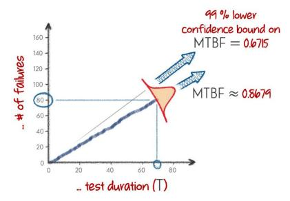
As you would expect, the *MTBF* 99 % **lower confidence bound** (0.6715 usage units per failure) is lower than the *MTBF* 'best guess' (0.8679 usage units per failure).
