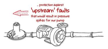
There are lots of examples of **fault containment** that range from voltage regulators through to filters. Each component has a different range of options based on the dominant **failure mechanisms** (**VITAL FEW**).
