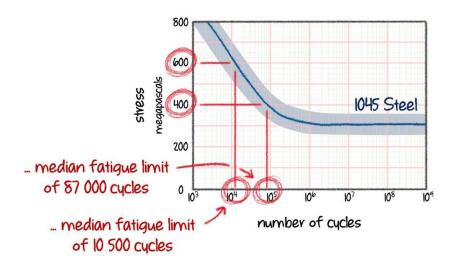
Remember, the horizontal axis above is in a **logarithmic scale**. So let's say our strut is exposed to 7 500 cycles at 600 MPa and 30 000 cycles at 400 MPa
