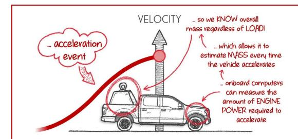
Ford vehicles are able to constantly estimate vehicle (and load) mass every time the driver presses the accelerator. So even if it is loaded, unloaded, takes on passengers and so on, the on-board computer has a really good understanding of vehicle (and load) mass ... all the time.
