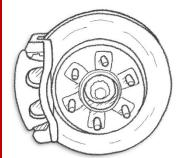
Brake pads convert kinetic energy to thermal energy when the calipers clamp them to the spinning rotor. This slows our vehicle down.
