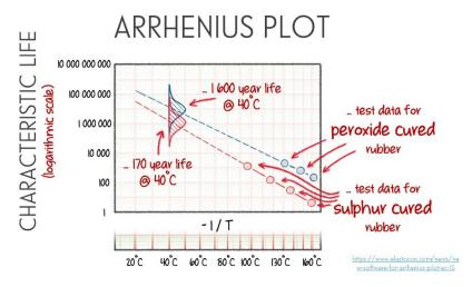
The data on the bottom right-hand corner of the chart doesn't take very long to gather as the temperature has been increased. We can see that because the data creates a straight line, the **Arrhenius model** appears to be a good fit.
