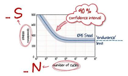
You can see that the horizontal scale of the 'S-N' chart above is **logarithmic**. And because fatigue cycles to failure is described by the **lognormal distribution**, the *logarithm* of fatigue cycles to failure should be described by the **normal distribution**.
