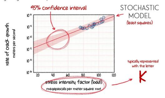
A basic **stochastic model** has been applied (with **confidence bounds**). It essentially revolves around an assumption that the **logarithm** of the rate of crack growth is proportional to the stress intensity factor.
