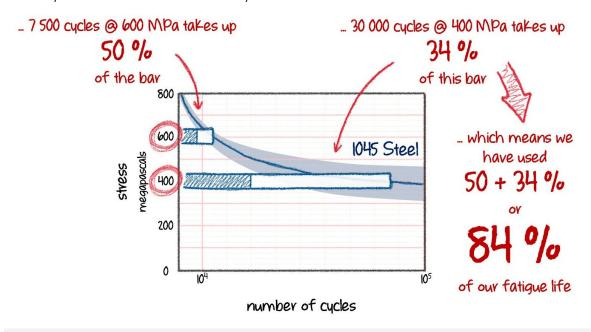
This approach to trying to combine fatigue models at different stresses is called **Miner's Rule**. Note that this is called 'rule' because it is an unproven hypothesis.
