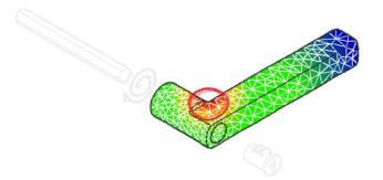
We know (from experience) that the **lognormal distribution** does a good job of modelling fatigue failure. As a fatigue crack grows bigger, it concentrates more stress at the crack tip. So the crack grows faster in a 'multiplicative' way.
