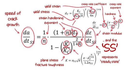
And when we combine this **mechanistic model** with the observed data we get ...
