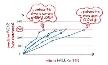
This is where our understanding of the wear mechanism (or any other failure mechanism) becomes incredibly useful. We know that the amount of brake pad material that is worn away is proportional to the amount of kinetic energy that is transferred to thermal energy. And all we need to know for each braking event is the start and finish velocities, along with the mass of the vehicle (with any load).
