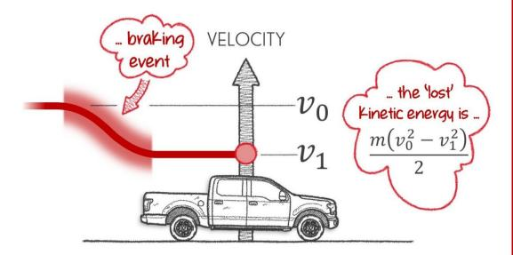
Vehicles are getting smarter and smarter these days. On board computers can measure the initial and final speeds of each braking event. But the vehicle mass ... with any load?
