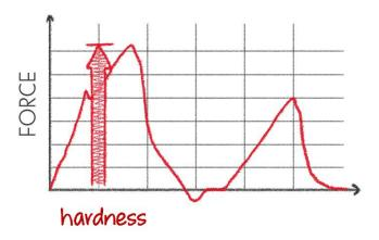
The second metric is **cohesiveness** which measures the ability of the bread to not be damaged during the test. The less damage the bread incurs, the closer the size of two areas under the force profile for each movement will be.
