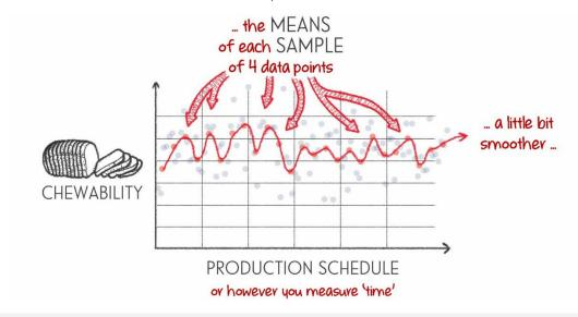
The next measure is **dispersion**. A very simple way of estimating **dispersion** for each sample is finding the **range** of each **sample**. The **range** is simply the difference between the highest and lowest **process** or **product characteristics** (**chewability**).
