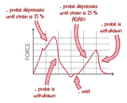
Three key metrics can be calculated from this profile. The first is **hardness**, which is the maximum force the bread exerts on the probe as it is being moved down the first time.
