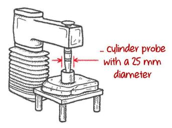
The texture analyzer has the ability to very slowly move an attached probe up and down and measure the smallest of forces that the probe experiences. In the illustration above, two slices of bread are being tested together.
