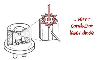
The element in the image above is a semiconductor that is not based on silicon. Instead, it is based on gallium aluminium arsenide (AlGaAs). This becomes a Light Emitting Diode (LED). There are mirrors on the surface of the semi-conductor to create a laser cavity. The laser is then emitted out the 'side' of the semiconductor in a controllable way.
