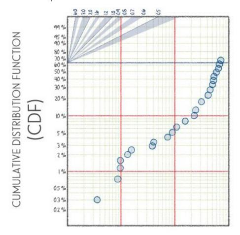
And we can work out straight away from this plot the nature of failure. We can tell that because the line of 'best fit' is steeper than the dotted line, the **shape parameter** ( $\beta$ ) is greater than 1 AND our product, system or service is wearing out.
