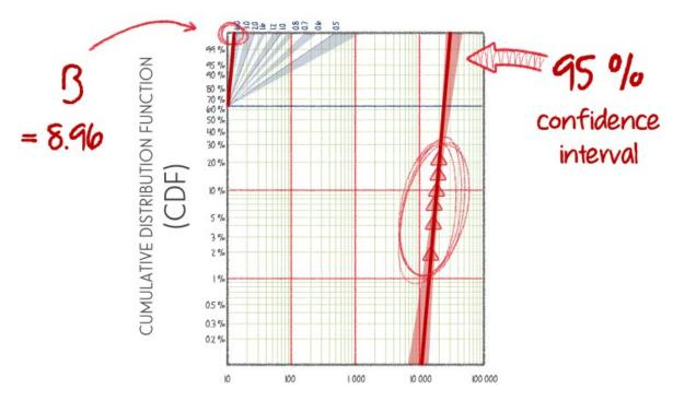
For this particular plot, the line of best fit has a slope of 8.96. This corresponds with the ' $\beta$ ' or shape parameter of the Weibull distribution that best fits the data.
