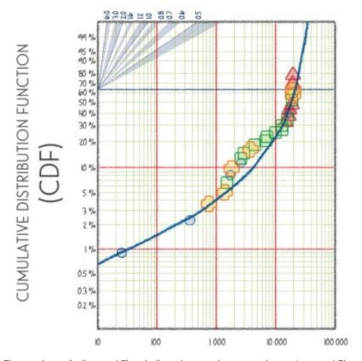
This is a basic 'bell curve.' The shallow slope at the start indicates 'wear-in.' The steeper slope at the end indicates 'wear-out.' And the bit in between shows 'constant hazard rate' failures.
