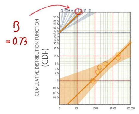
For this particular plot, the line of best fit has a slope of 0.73. Remember, this corresponds with the ' $\beta$ ' or shape parameter of the Weibull distribution that best fits the data.
