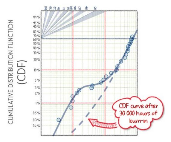
A burn-in of 30 000 hours is *very* long. For example, there are 8 766 in a single year. But burn-in can be accelerated in a controlled way where we might (for example) increase the temperature to create a burn-in test that is equivalent to 30 000 hours in a much shorter period.
