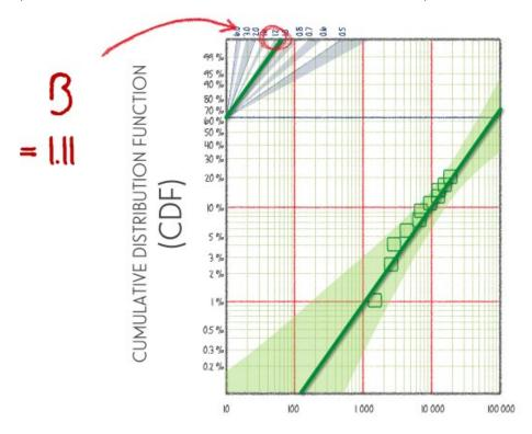
For this particular plot, the line of best fit has a slope of 1.11. Remember, this corresponds with the ' $\beta$ ' or shape parameter of the Weibull distribution that best fits the data.
