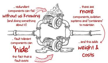
Redundancy comes at a cost - so we need to think about it. There is a hidden issue with redundancy - Common Cause Failure (CCF). Single faults often cause failure in primary and standby components, meaning we don't get the reliability improvements we hope for.
