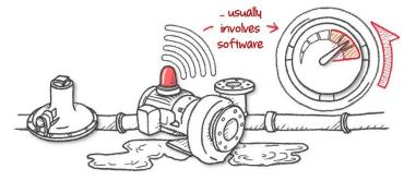
An example of reversion is an engine RPM limiter that enacts when a leak in the coolant system is identified. This will reduce the top speed of a vehicle but will allow the vehicle to continue operating. While **reversion** can be manual (as in, an operator manually detects a fault and adapts the use conditions accordingly), it is typically automated using sensors and software.
