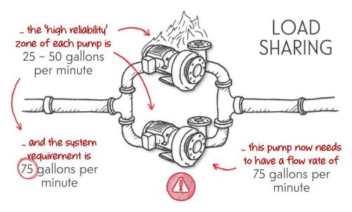
The system is required to pump 75 gallons per minute. Both pumps can have their service life extended by making sure that they pump somewhere between 25 and 50 gallons per minute. When both pumps are working, they need to pump at a rate of 37.5 gallons per minute for the. This means they both remain in a 'high-reliability' zone.
