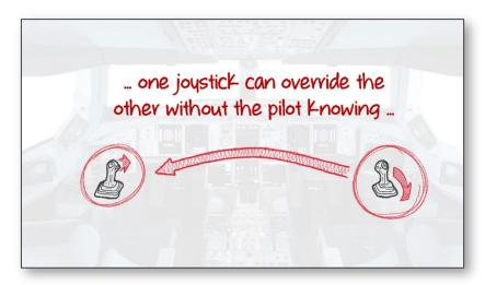
These controls are fundamentally different to the highly visible and connected control yokes of other airplanes.
