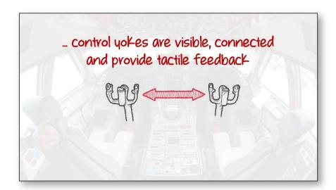
The Air France 447 copilot for whatever reason pulled 'back' on the side stick, pushing the nose of the aircraft up. This place it in a stall condition and it started plummeting toward the ocean. The other pilot was trying to push the nose down with his side stick – and he couldn't understand why the plane wasn't responding. By the time the crew realized what was happening – it was too late.
