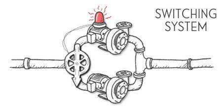
A **switching system** needs a switch mechanism that can recognize when the first pump **fails**, and then successfully **'switch**' the **standby pump** to an **'active**' state. This introduces additional ways the system can **fail** but can substantially increase system **reliability**.
