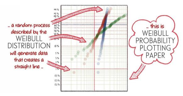
And that straight line can be used to estimate our **Weibull distribution parameters** directly. We know that because the **CDF** of any **Weibull** will be 63.212 % at the **characteristic life**. So we can find the **scale parameter** from the **Weibull plot** where the **CDF** is 63.212 %.
