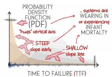
All the **PDF curves** in the previous illustrations (each one modelling a different **failure mechanism**) were all specific examples of the **Weibull distribution**. And ... they all had the same **mean** or **mean time between failure (MTBF)**. This further illustrates that just understanding the mean of the **random process** that is **failure** reveals very, very little about the **reliability characteristics**.
