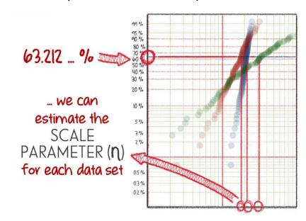
We can use the slopes of the lines of best fit to estimate the **shape parameter** of each process.
