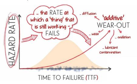
The PDF and hazard rate curves for a Weibull distribution with a shape parameter of 2 are illustrated below. This closely mimics some lognormal distributions.
