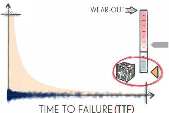
In fact, different products with different probability density curves for times to failure (like the compressor vane below) each have their own 'place' on the gauge that represents the extent to which something wears-in or wears-out.
