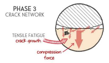
Eventually, this crack network will reach the surface, or a surface crack will grow to be relatively 'large.' From above, this will create a 'v' shape surface crack.
