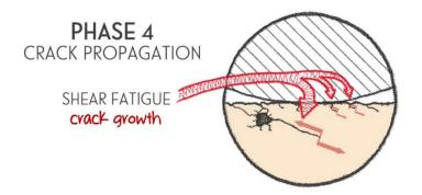
This crack initially grows at a shallow angle (approximately 35°) to the surface. Once the crack is deep enough, it then turns and travels parallel to the race surface. Eventually, the shearing forces will cause the crack to go back to the surface.
