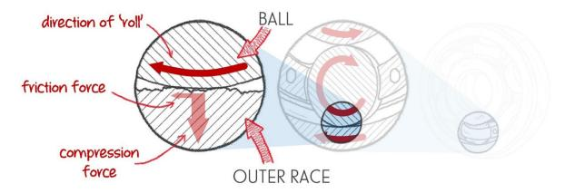
The first step in spalling is actually plastic deformation or smoothing of the race surface. This absorbs energy and otherwise protects the race material
