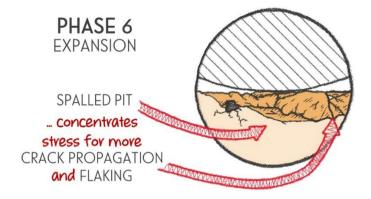
When enough material has flaked away, the ball bearing will vibrate excessively, be noisy, and generate a lot of heat that will either directly or indirectly lead to catastrophic failure.
