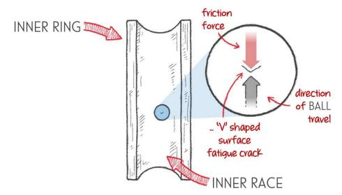
This then leads to another type of fatigue crack that grows not due to tension, but to shear. That is where one side of the crack tip is being 'pulled back' while the other side is being 'pushed forward.'
