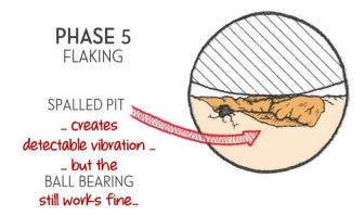
These pits will be visually detectable (for the first time) if the ball bearing can be accessed.
