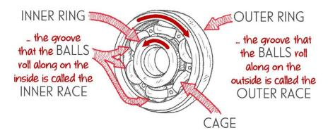
Ball bearings are designed to minimize the friction a rotating shaft experiences when it is supported within a machine. Because freely supported balls are the only physical connections between the inner and outer rings, it is very difficult for 'torque' to transferred. Every time torque is generated, the balls simply roll. This greatly minimizes any frictional forces.
