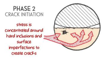
Because the balls repeated roll over the surface, the tensile stresses cycle that allows fatigue cracking to occur.
