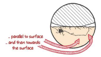
Because the crack has reached the surface, chunks of the race material can now break free.
