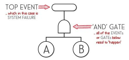
The circles with the letters 'A' and 'B' in them represent 'Basic Events' corresponding with the failures of pumps 'A' and 'B' respectively.
