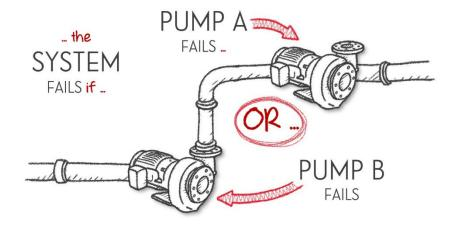
A Fault Tree can model this system using an 'OR' gate ...
