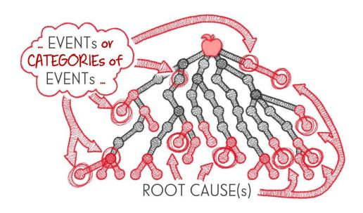
Each branch is what we call a 'Causal Chain' which is a sequence of cascading events where one event becomes the trigger for the next event. The first event in this Causal Chain is the Root Cause, while failure is the last or ultimate event.
