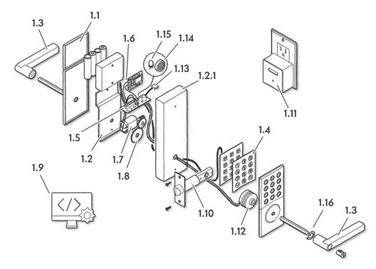
At the 'heart' of the smart lock is the electric motor that is controlled by the Printable Circuit Board (PCB) and the gearset it turns.
