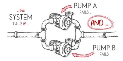
A Fault Tree can model this system using an 'AND' gate ...
