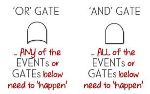
To understand how these gates work, let's look at a two pump 'Parallel System' where one pump is redundant.
