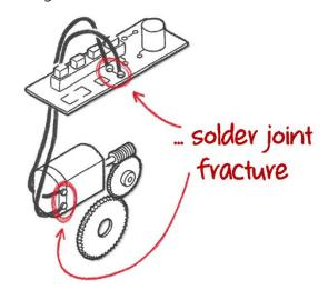
Is 'solder joint fracture' a Root Cause of failure? NO. Because we can't change this. This is a symptom of something we need to do different. Simply resoldering these joints won't prevent whatever issue exists in our design from causing this failure again in the future.
