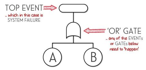
Fault Trees, like Ishikawa Diagrams, allow us to go down one layer at a time. For example, we might brainstorm the following layer #1 'Input Events' and 'Undeveloped Events' as part of Root Cause Analysis for our motor cable junction failure.
