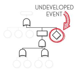
There are also 'Input Events' we represent with rectangles that allow us to label what each part of our Fault Tree represents. For example, an 'Input Event' might be 'Power Supply Failure' because the elements of the Fault Tree beneath it represent different ways that the power supply could fail.
