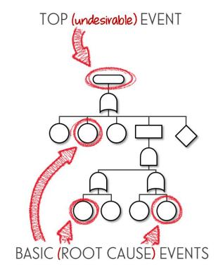
So the diagram above represents potential Root Cause with circular or round shapes that are called 'basic events.' The structure and layout of the Fault Tree shows us what Basic Events can result in the Top or 'undesirable' event which represents the failure event which triggered the Root Cause Analysis.
