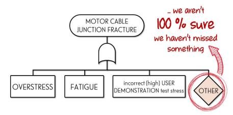
We then focus on one of the 'Input Events,' such as 'Overstress' and then brainstorm layers until we arrive at events that we believe satisfy the definition of being a Root Cause. We then replace the rectangular shapes of 'Input Events' with the round, circular shapes of 'Basic Events' to show that those events now need to become the basis of generating potential Corrective Actions.
