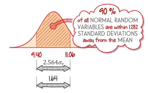
This allows us to calculate the second **lognormal distribution** parameter,  $\sigma_{ au}$  ...
