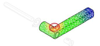
We know (from experience) that the **lognormal distribution** does a good job of modelling fatigue failure. As a fatigue crack grows bigger, it concentrates more stress at the crack tip. So the crack grows faster in a 'multiplicative' way.
