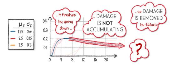
This is not possible for a **failure mechanism**. If a **failure mechanism** is based on the accumulation of damage, it never gets to a stage where the accumulation of damage stops.
