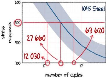
What we are going to do now is use the normal distribution (noting that this chart uses a logarithmic scale). So we can't use the cycle numbers above – we need to use the logarithms of these numbers
