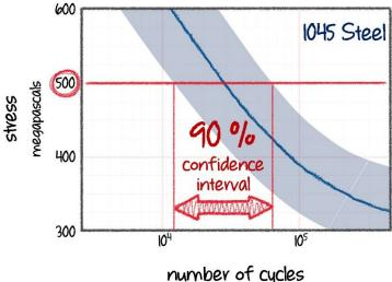
We can identify the boundaries and mid point of this interval using this chart.
