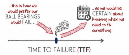
But this is not reality. In practice, ball bearings will **fail** at different times. But just because something is **random**, doesn't mean its unpredictable.
