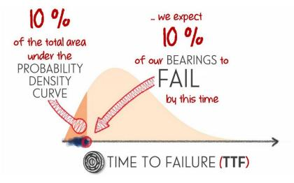
We are almost always only interested in understanding when the first 'small fraction' of products or components will **fail**. We typically want to replace most things before they **fail**, as **failure** is much more expensive (and potentially damaging) then a scheduled replacement.
