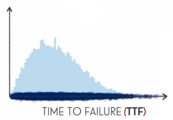
If we test an INCREDIBLE number of **ball bearings**, we would get a **histogram** with the bars are so small that they create a smooth shape (perhaps called the **ultimate histogram**). The curve on top of this shape has a special name ...
