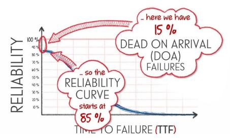
This is a common problem for products, machines and systems that deploy in arduous conditions. And 'arduous' conditions can include product mishandling by delivery truck drivers. So if 15 % of products (like small satellites) suffer **DOA failures**, then their **reliability curves** need to start at 85 % instead of 100 %.
