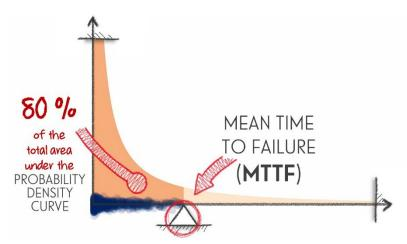
So even though the weird **ultimate histogram** shape above is perfectly balanced on the **mean** (**MTTF**), 80 % of its area is on the left. This is because the remaining 20 % on the right extends so far out that it creates more 'leverage' to create this perfect balance even though this only accounts for a small fraction of this area.
