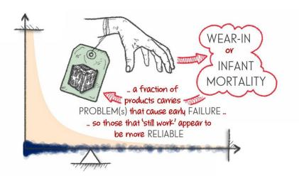
Products with lots of **defects** that **wear out** have **ultimate histogram** shapes that hug the vertical axis as shown above. And these **defects** include the seemingly ever-present manufacturing problems, **assembly** or **installation error**, **interface issues** (between components), **damage** during transit or launch, and **software bugs**. This weird shape has an 'interesting' **mean** or balance point.
