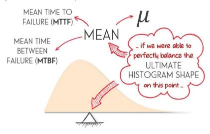
The symbol ' $\mu$ ' is a Greek lowercase letter that is pronounce 'mu.' Because the **mean** is just the balance point of the **ultimate histogram** shape, it has no physical meaning. But the **mean**, **Mean Time to Failure** (MTTF), or **Mean Time between Failure** (MTBF) if our product is repairable is often used to 'represent' **reliability**. The **mean** is NOT **reliability**.
