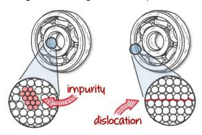
A **dislocation** involves neighboring rows of metal atoms that don't line up perfectly. Both **impurities** and **dislocations** are invisible microscopic **defects** that create lots of tiny structural weaknesses that differ between **ball bearings** that look identical to us. So ball bearings will fail in slightly different ways at perhaps very different times.
