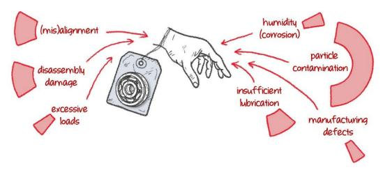
Experience has shown that manufacturing **defects** (like **impurities** and **dislocations**) play a small role in how long each **ball bearing** lasts. How we treat our **ball bearings** (lubrication, maintenance, correct alignment and so on) is much more important.
