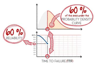
The **probability density curve** aligns with how our brains like visualize **randomness**. The height of the **probability density curve** at a particular **TTF** represents how likely it is for our product to **fail** at that **TTF**.
