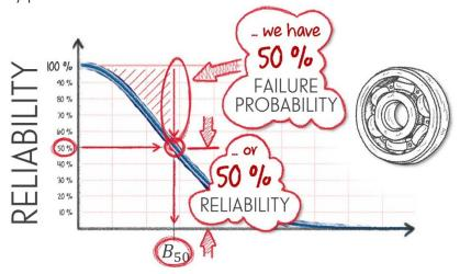
We call the time when a product has **50** % **reliability** (or when we expect half our products to have **failed**) the  $L_{50}$  **life** or  $B_{50}$  **life** if the component is a **ball bearing**. And all **reliability curves** 'head' in the same direction as products get older.
