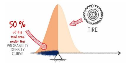
This is how our human brains prefer visualizing **randomness**. We expect half of all tires to **fail** by the **mean** (**MTTF**). And just to confirm, the balance points for the small satellite (on the previous page) and the rubber tire **ultimate histogram** shapes are in exactly the same place.
