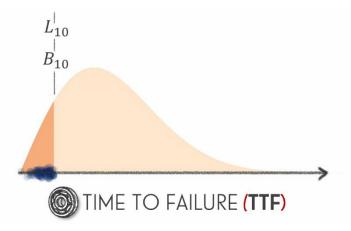
Most (90 %) of the area under the **probability density curve** is to the right of the  $L_{10}$  or  $B_{10}$  life. This represents the fraction of **ball bearings** that are still working at the  $L_{10}$  or  $B_{10}$  life.
