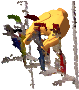
Figure 3: Raw 3D sensor data is, by its nature, incomplete and noisy, as seen in this side rendering of point data for objects on a shelf.
