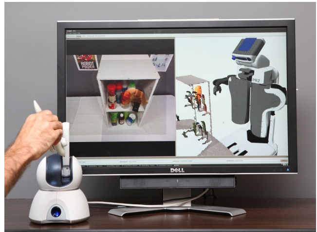
Figure 1: An operator using a haptic device to direct a robot performing a grasping task. The algorithm presented is fully 6-DOF, although the user-study was conducted using a 3-active, 3-passive DOF device that rendered forces only.
