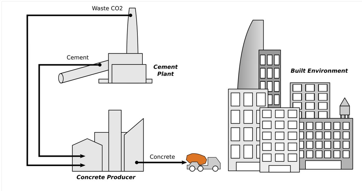
**Figure 2. Circular economy principles for concrete production – Use waste CO<sub>2</sub> from cement plants to create better concrete**
