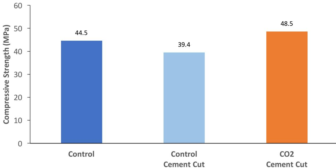
**Figure 3. Ready Mixed Concrete Production – 28 day compressive strength of control batch, batch with reduced cement, and batch with reduced cement produced using CO<sub>2</sub>**
