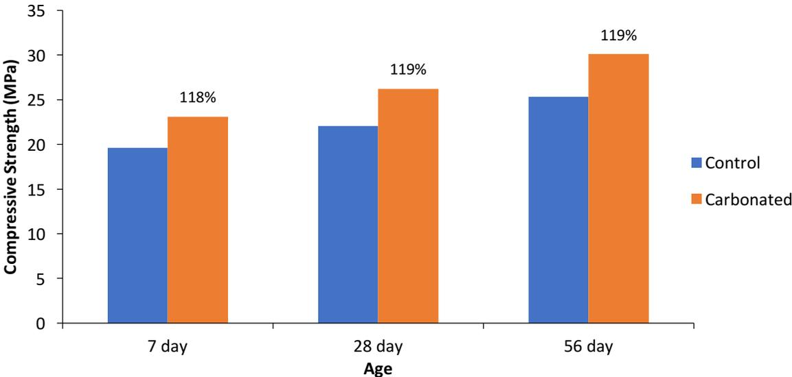
Figure 3. Compressive Strength of concrete masonry units produced with and without a CO<sub>2</sub> addition
