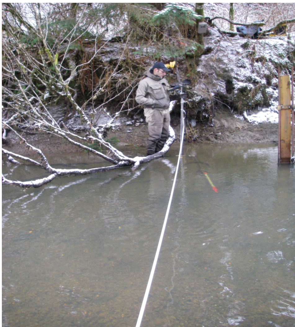
Appendix C1.—Looking across at streamgage 11701 on November 19, 2008 at a discharge of 30 cfs. The gage housing is located on the streambank. The wellhead (with an orange tip) contains the transducer and is shown extending from the bank underwater. The staff gage is shown just upstream of the tagline
