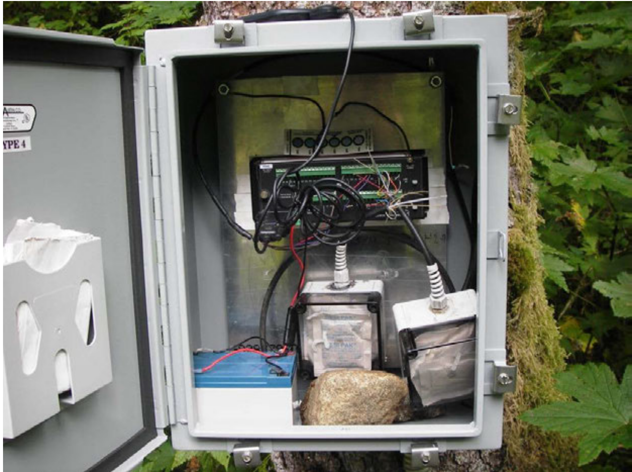
Appendix C3.—Metal enclosure attached to a tree near streamgage 10302 that housed the first data logger and battery used during the project. Note the wiring that was required from both the transducer and battery to the data logger.
