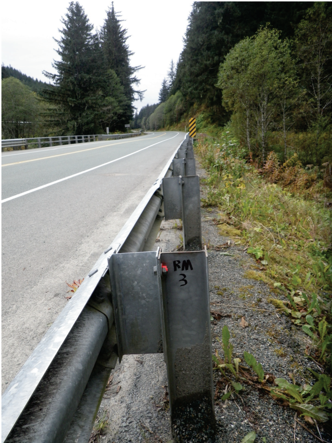
Figure 8.—Third water surface elevation marker (RM3) ;bolt on guardrail seen looking south along Glacier Highway.
