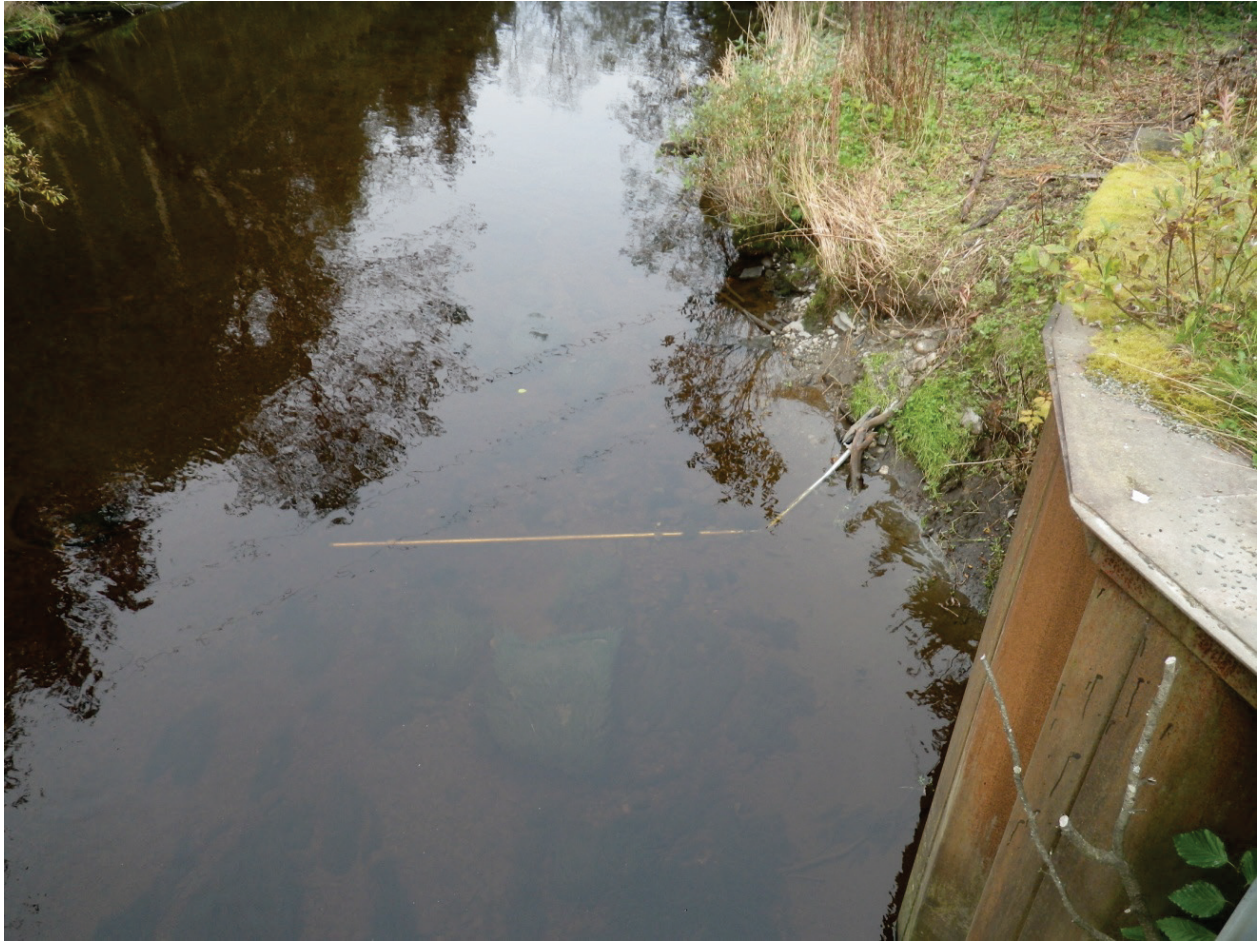
Figure 4.–Looking downstream from Glacier Highway bridge at ADF&G Streamgage 13601, with pressure transducer house in pipe secured to stream bank with brackets and rebar.
