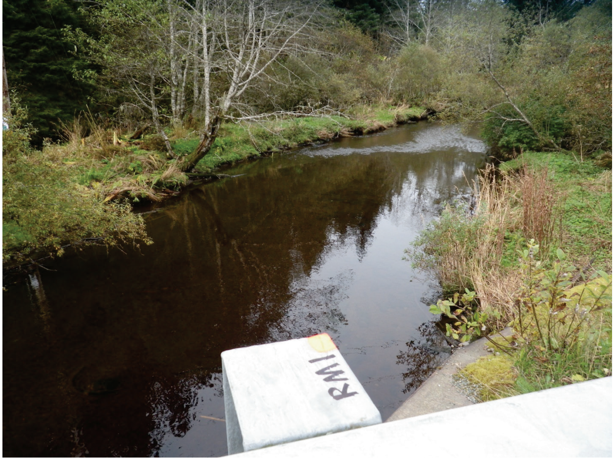
Figure 6.–Looking downstream from Glacier Highway bridge showing reference mark (RM1) for comparative water surface elevation measurements.
