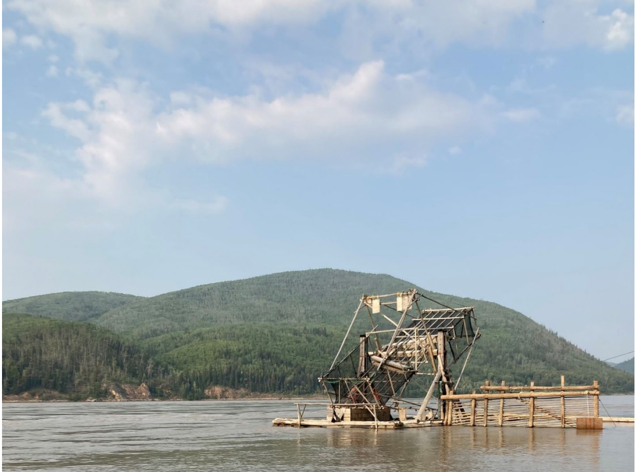
Figure 2.3. Fish wheel with baskets lifted out of the water located at the Rapids sampling site.
