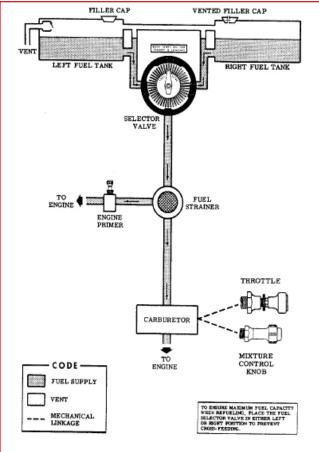
172 Fuel System (Standard & Long Range) with vented fuel feed
