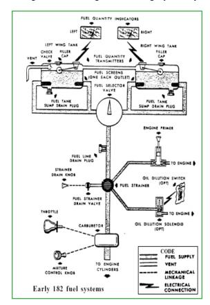
from the left tank. This means that there will not be fuel flow interruption to the engine even if the left tank were to go dry with the fuel selector in the 'BOTH' position.
