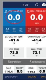
All of the pressures and temperatures will be assigned based on the previous session assignment. Note: The readings can be changed (i.e. switching high side module to low side) by clicking on the respective readings on the screen.
