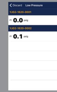
Assign the P51-TITAN that is connected to the low-side of the system. Repeat this process for the high-side pressure and temperatures.
