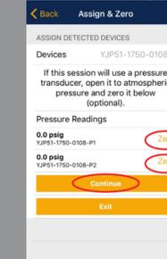
Click "Zero" to zero the pressure readings before connecting to the system. Click "Continue."
