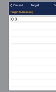
To assign a subcooling target, click on the Subcooling Target "—" and assign the target subcooling values.
