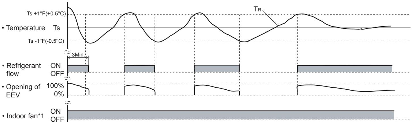
Ts : Corrected setting temperature      TR : Corrected room temperature
