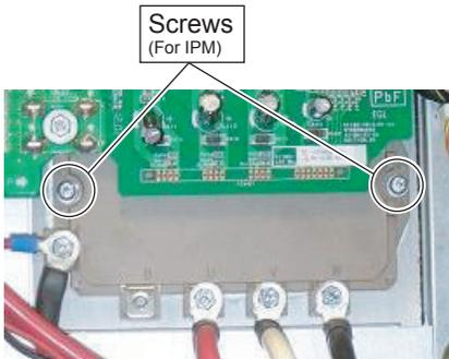
Remove the 2 mounting screws.
