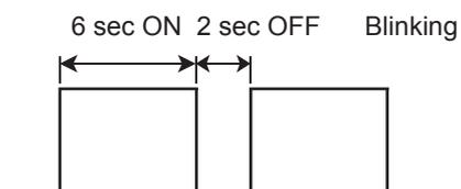
Indoor fan : Same operation before oil recovery operation in cooling operation or dry operation.(Heating operation: Stop)
