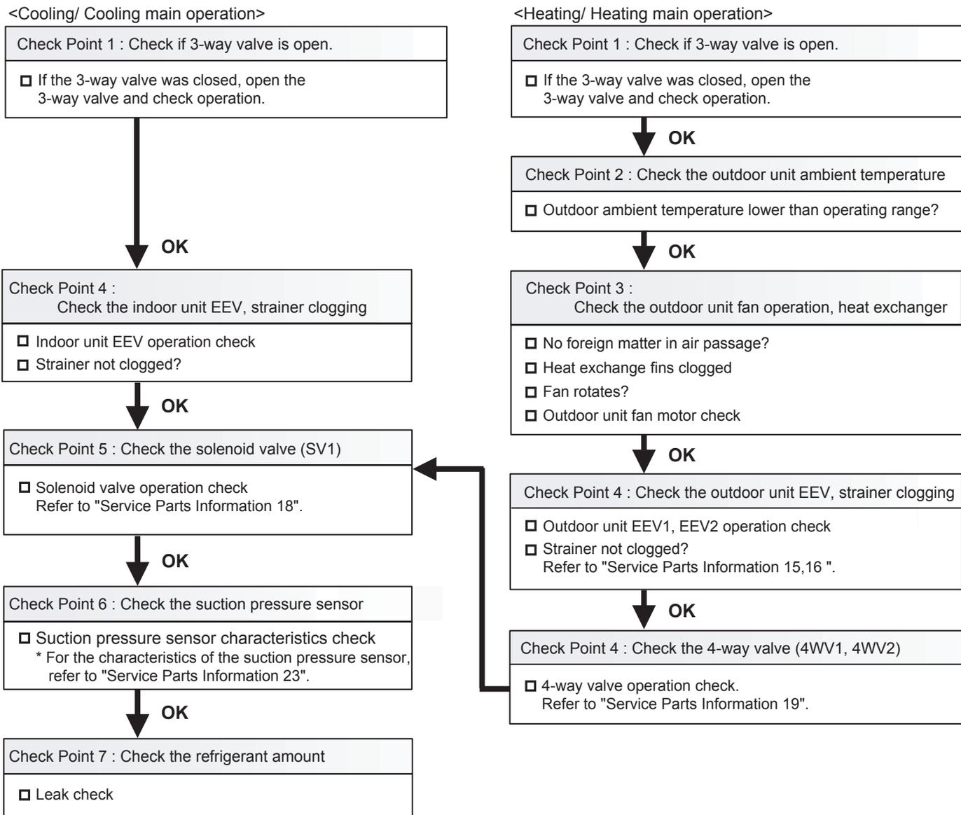
After fixing the problem and for canceling the Error, Error Reset (F3-40) will be required after power reset
