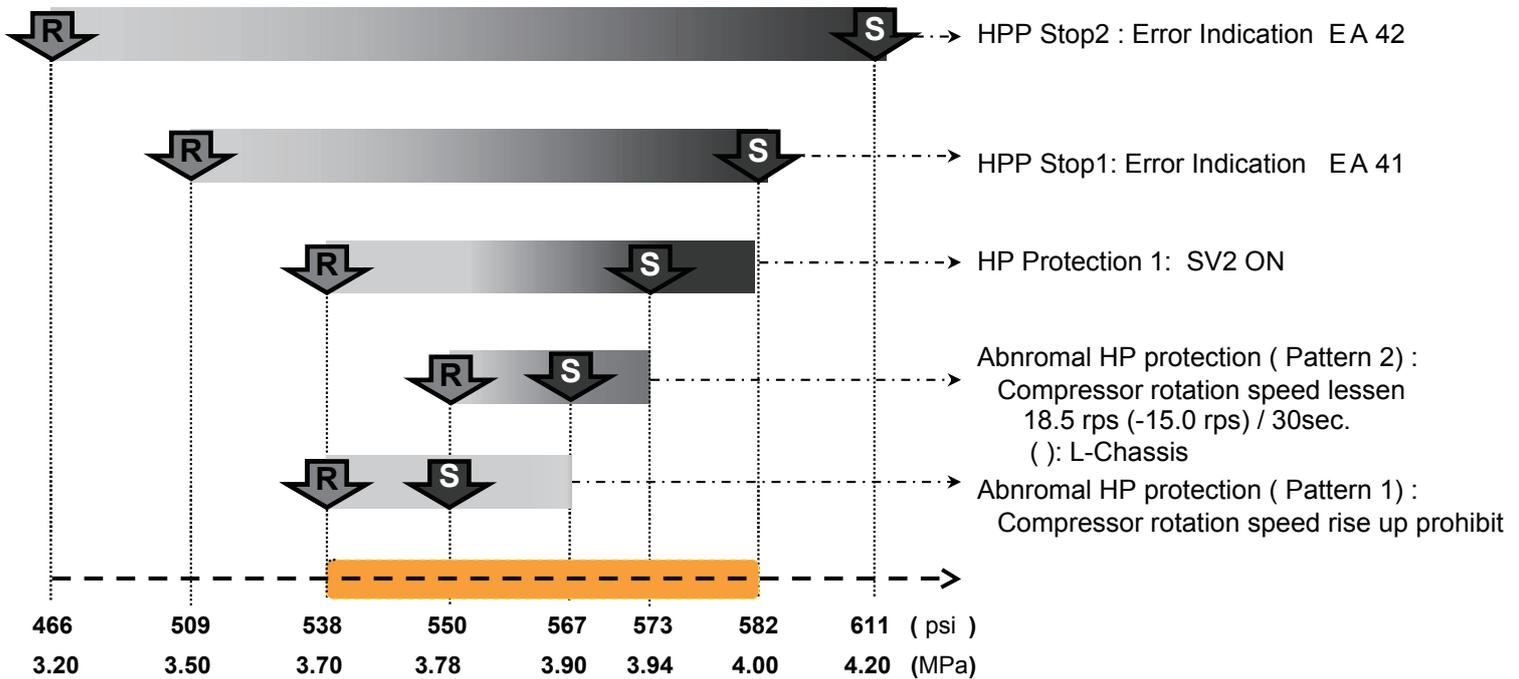
Note: Target pressure controlling will be cancelled when the operating pressure is in the range of orange.
