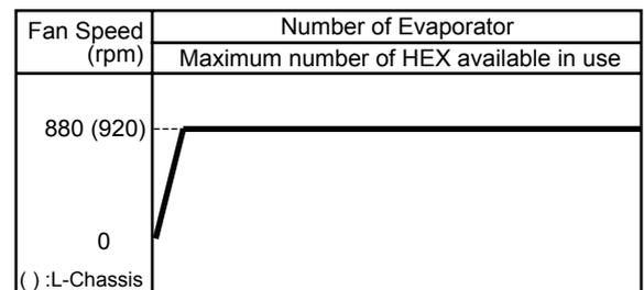
(3) Cooling Main / Heating Main (In case of 3 outdoor units connection)
