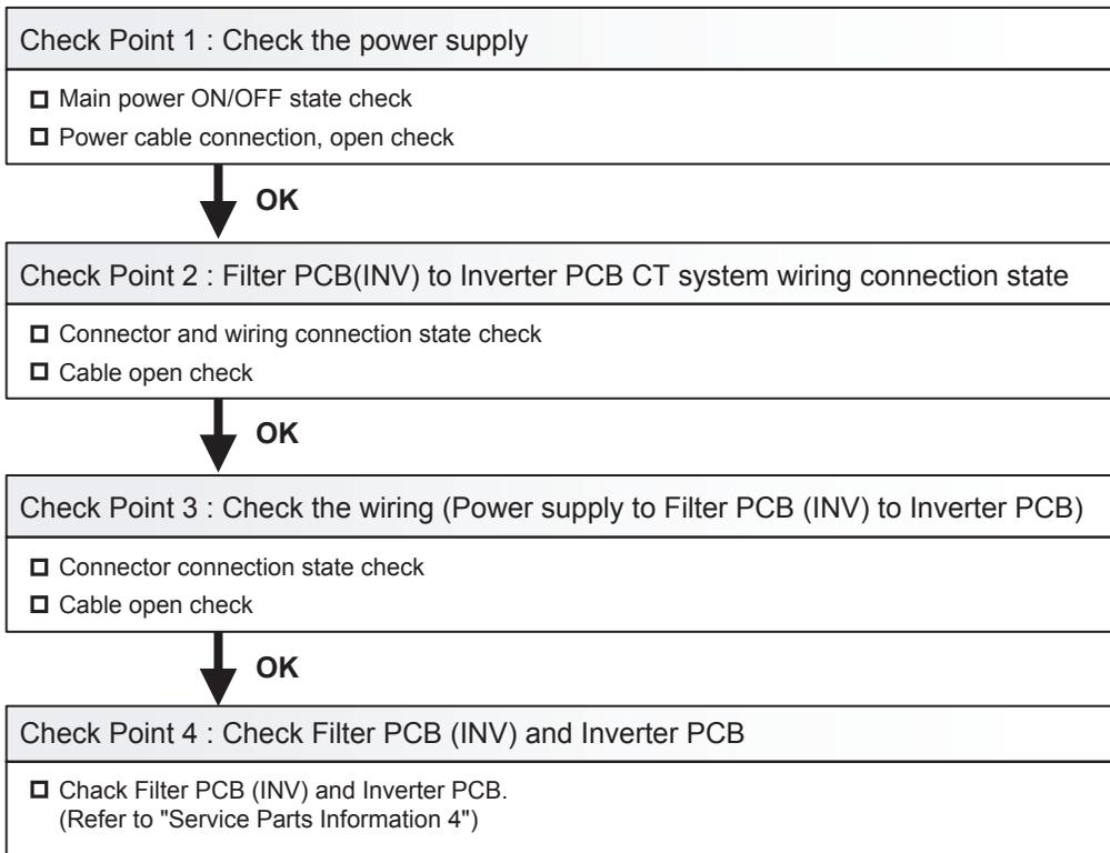
After fixing the problem and for canceling the Error, Error Reset (F3-40) will be required after power reset
