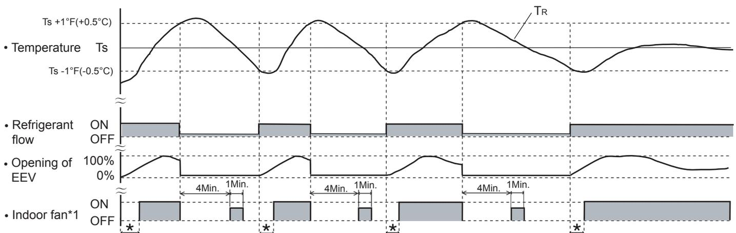
Ts : Corrected setting temperature      TR : Corrected room temperature
