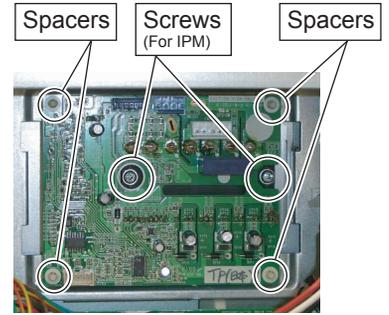
Remove the 2 mounting screws and the spacers.
