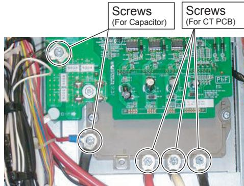
Remove the 5 mounting screws and codes.
