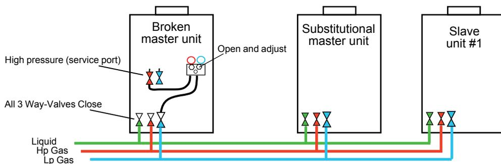
Connect the high pressure service port of the broken master unit and the low pressure pipe of the broken master unit by pressure gauge.
