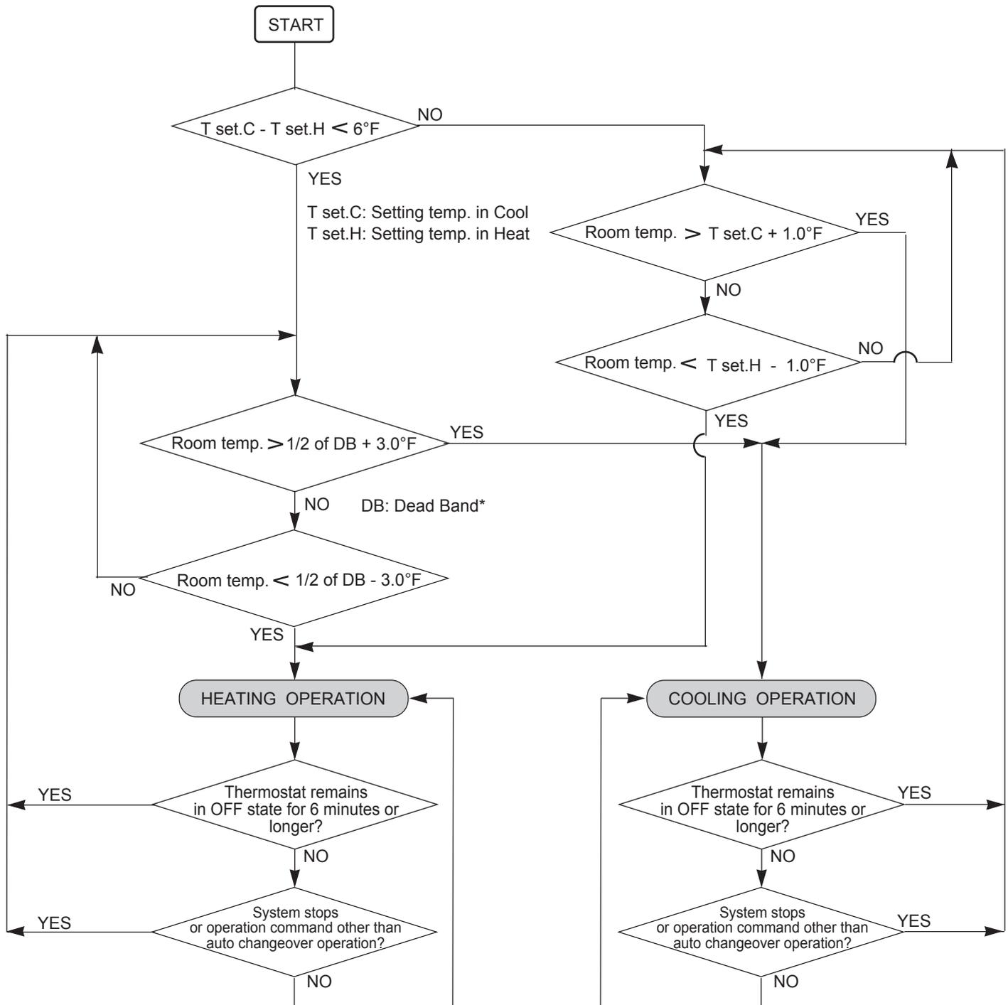
\*Dead Band(DB) means between T set.C and T set.H, however the setting parameter of Dead Band always has a priority.
