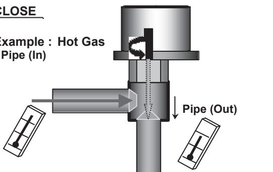
If it is open, it has no temp. difference between Inlet and Outlet.
