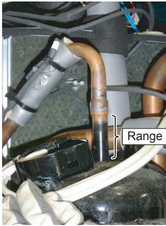
Cut the Discharge pipe in this range.
