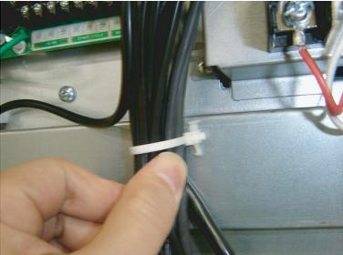
Loose or remove the cable ties. (3 places)
