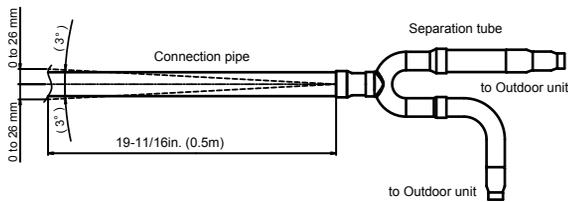
• Like the figure, adjust the pipe angle so as to be within 3-degree angle.
