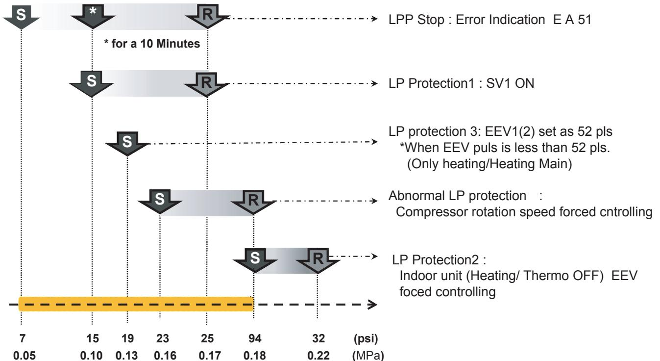
Note: Target pressure controlling will be cancelled when the operating pressure is in the range of orange.
