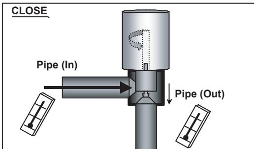
If it is open, it has a temp. difference between Inlet and Outlet. Outlet temp. is near Low-pressure saturated temp.
