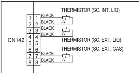
Sub-cooling heat ex. gas outlet temp. sensor (CN142: 7-8)
