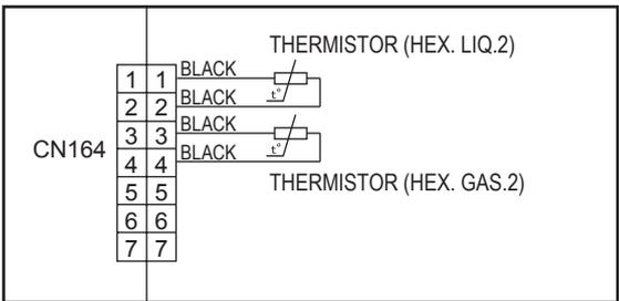
Heat ex.2 liquid temp. sensor (CN164: 1-2)
