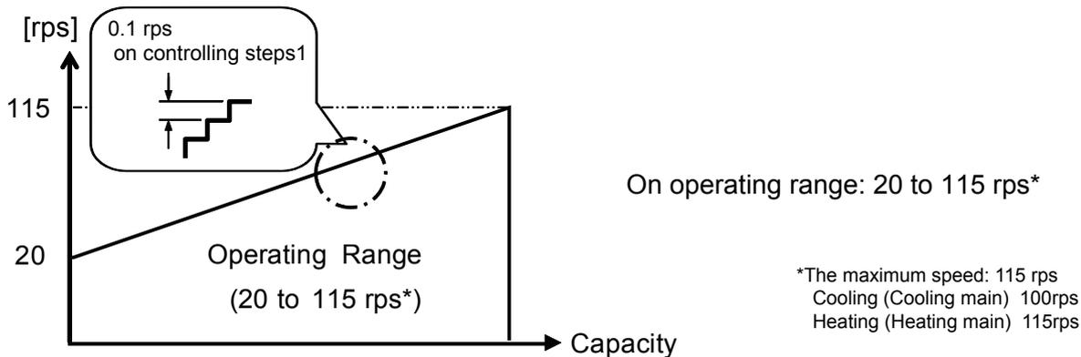
By combining the operation of inverter compressors, the amount of required refrigerant circulation according to cooling and heating load can be supplied from compressor efficiently.
