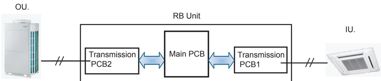
Main PCB: Pulse signal communication between Transmission PCB1 and Transmission PCB2
