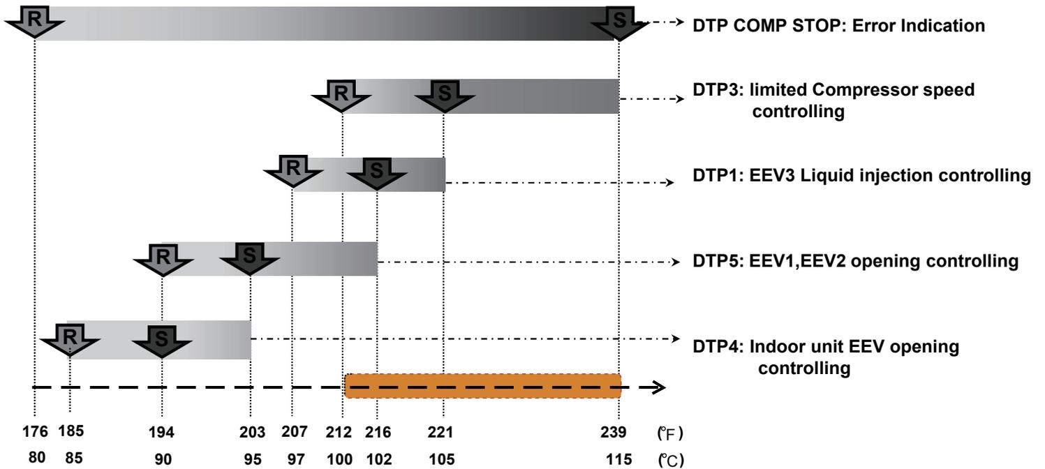
Note: Target pressure controlling will be cancelled when the temperature is in the range of orange.
