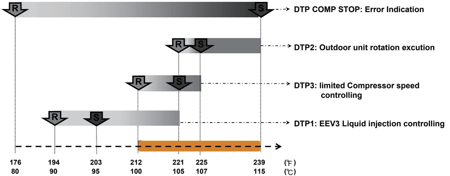
Note: Target pressure controlling will be cancelled when the temperature is in the range color orange.
