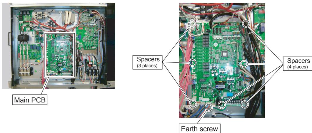
Remove the connectors and earth screw.
