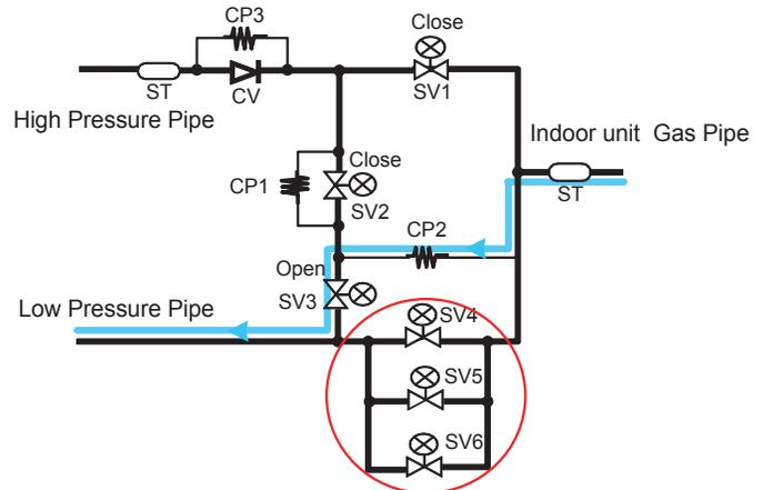
When SV4, SV5 SV6 internal blockage or Close position, the refrigerant flow will be lessened,
