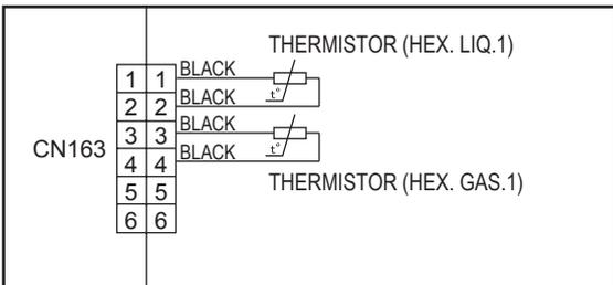
Heat ex.1 liquid temp. sensor (CN163: 1-2)
