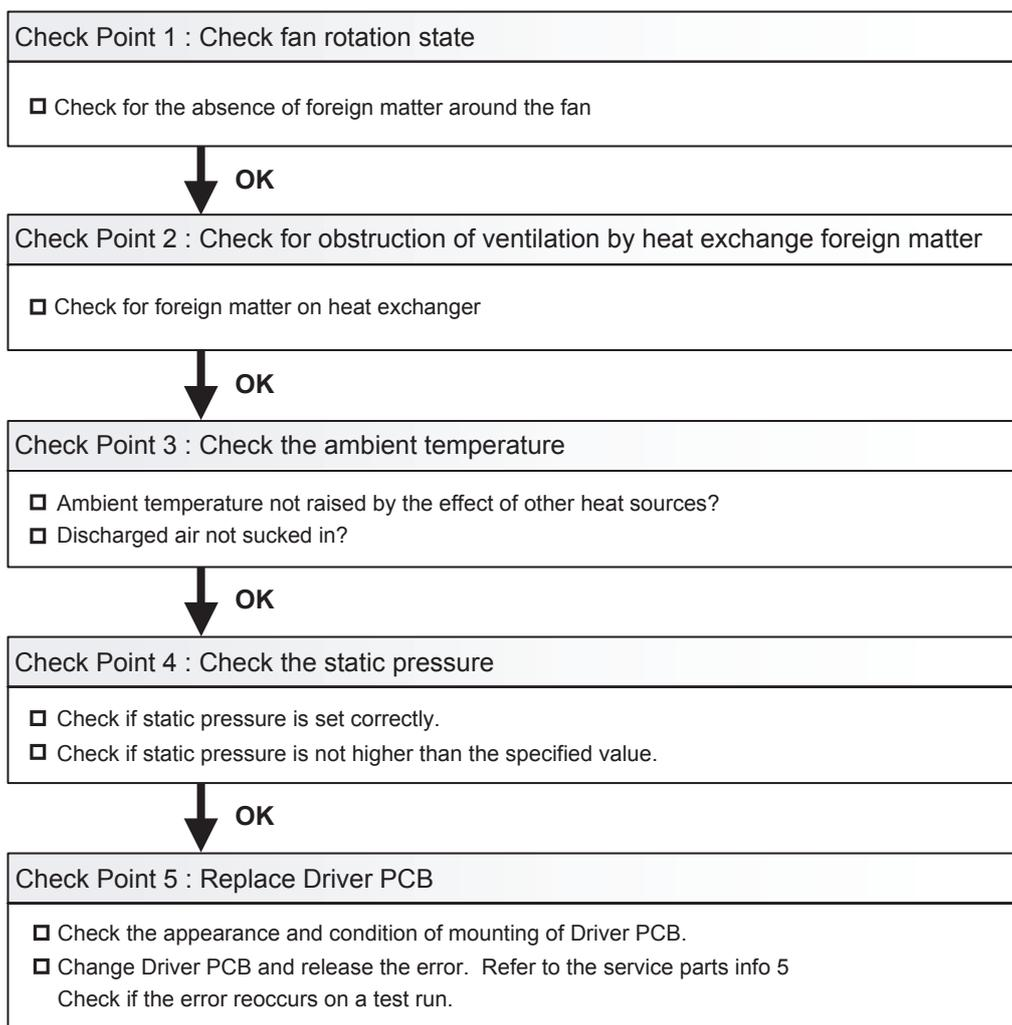
After fixing the problem and for canceling the Error, Error Reset (F3-40) will be required after power reset
