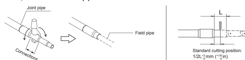
NOTE: Insert the field pipe firmly until it touches the joint pipe (Branch kit).
