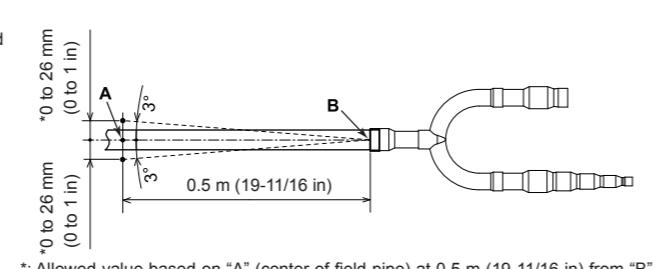
\*: Allowed value based on "A" (center of field pipe) at 0.5 m (19-11/16 in) from "B" (junction of the branch kit).
