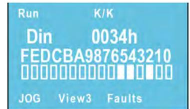
**View Screen 4:** This screen displays the status of the multi-function (digital) outputs in hex format. Solid boxes indicate that the output is active.
