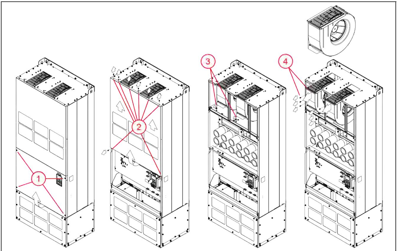
1. Remove four screws and remove the lower front cover. When replacing screws, tighten to a torque of 12 to 14 in. lbs. (1.37 to 1.57 Nm).
