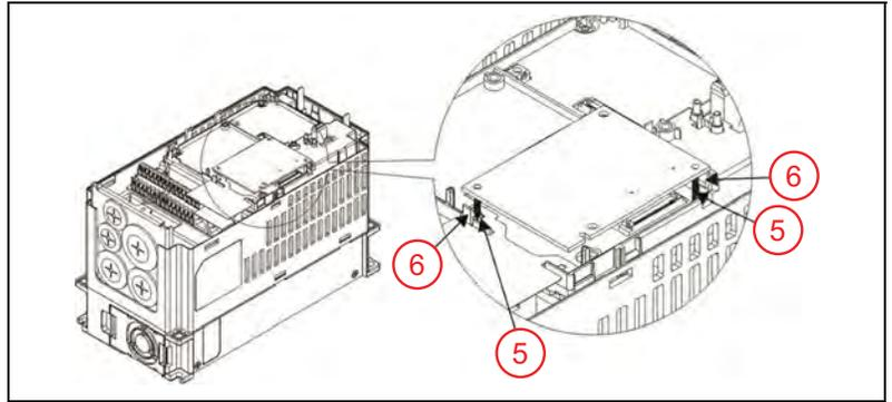
7. When clips are secure, install retaining screws and tighten to a torque of 6-8 kg-cm / 5.2-7 lb-in. / .59-.79 Nm.
