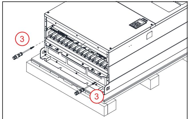
4. Install the conduit box to the drive using the following screws and nuts tightened to a torque of:
