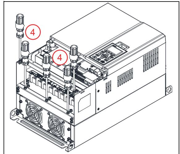
5. Install the conduit box with five screws. Tighten to a torque of 24-26 kg-cm / 20.8-22.6 lb-in. / 2.4-2.5 Nm.
