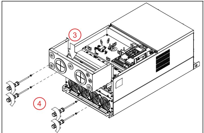
5. Install the conduit box cover using four screws from step 2.
