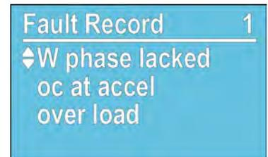
**NOTE:** Fault records can also be located through [PROT-51 to 56], or by pressing **Menu/Back/Down/Fault**.
