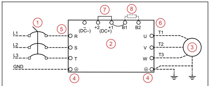
Use ring type terminals for the VFD power wiring.
