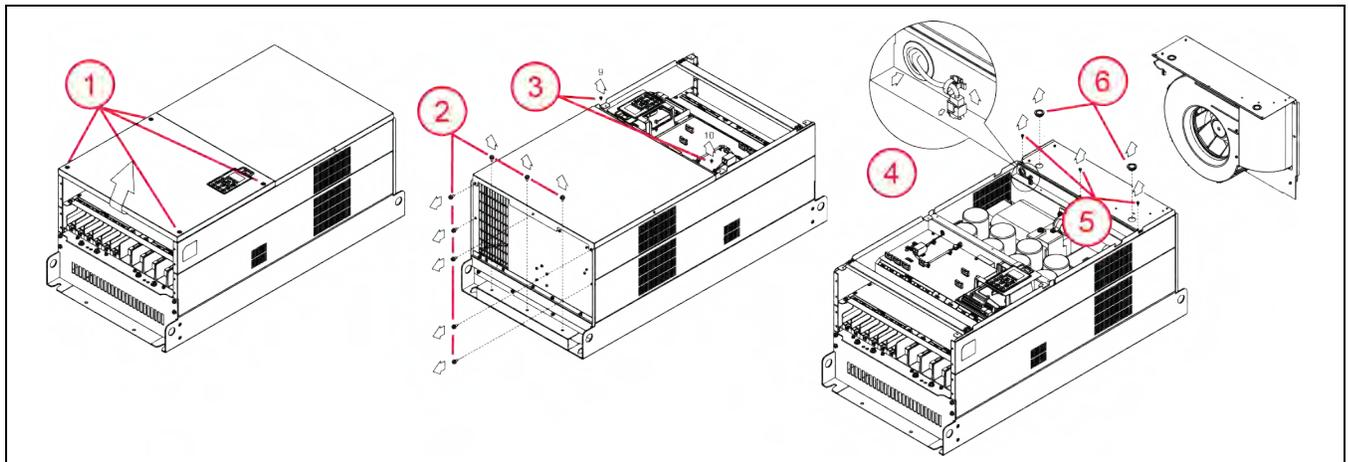
1. Remove four screws and remove the lower cover. When replacing screws, tighten to a torque of 10.4 to 13 in. lbs. (1.18 to 1.47 Nm).
