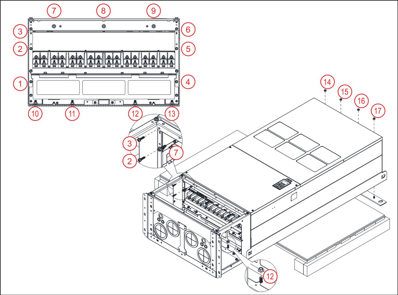
5. Replace the covers and screws removed in Step 1 to the original locations. Tighten to a torque of 35-45 kg-cm / 30.3-39 lb-in. / 3.4-4.4 Nm.
