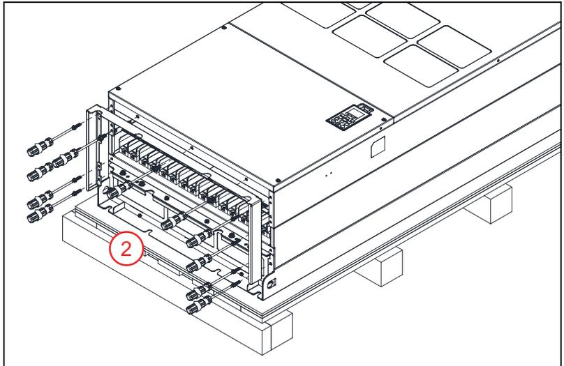
3. Fasten the M6 screws to two locations. Tighten screws to a torque of 35-45 kg-cm / 30.3-39 lb-in. / 3.4-4.4 Nm.
