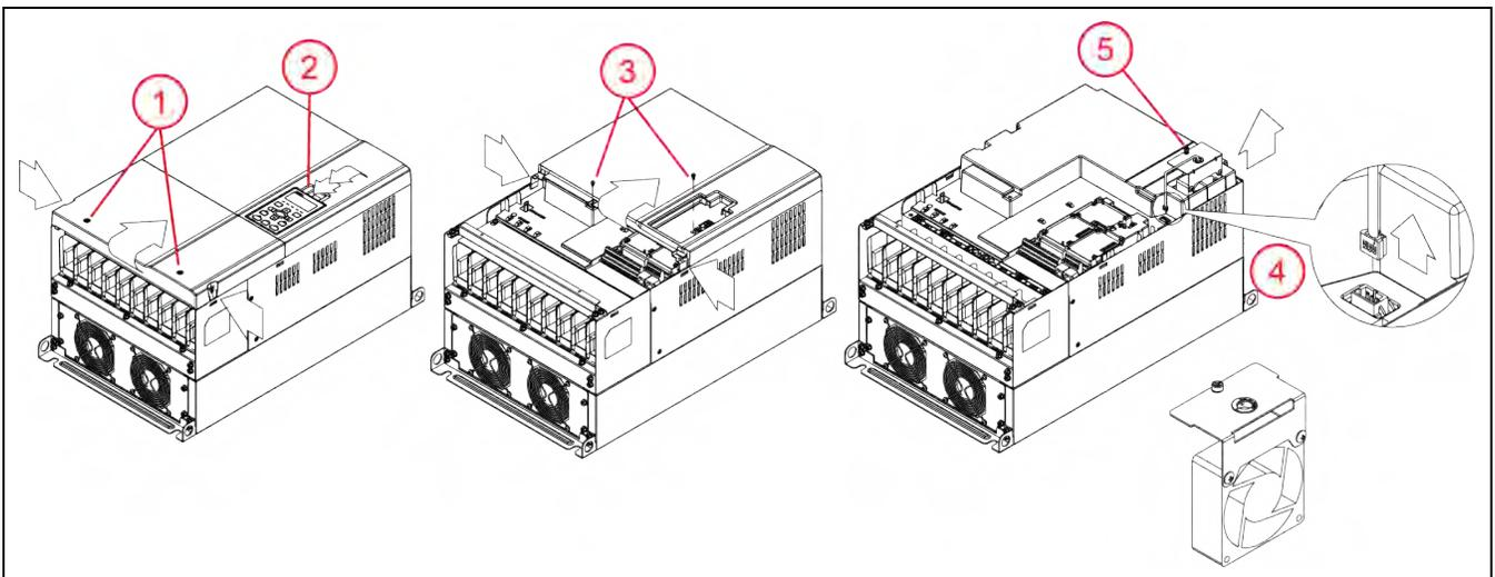
1. Remove two screws and press the tabs on both sides to remove the lower cover. When replacing screws, tighten to a torque of 10.4 to 13 in. lbs. (1.18 to 1.47 Nm).
