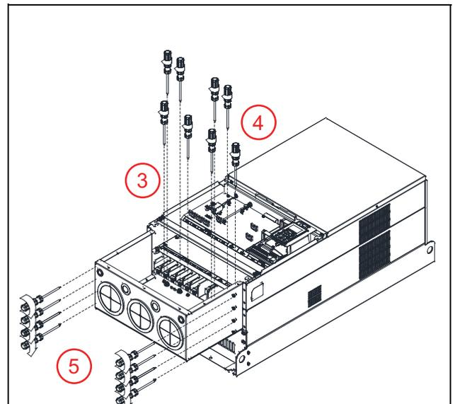
6. Set the conduit box cover on the conduit box and slide it toward the conduit knockouts. Tighten the screws to a torque of 24-26 kg-cm / 20.8-22.6 lb-in. / 2.4-2.5 Nm.
