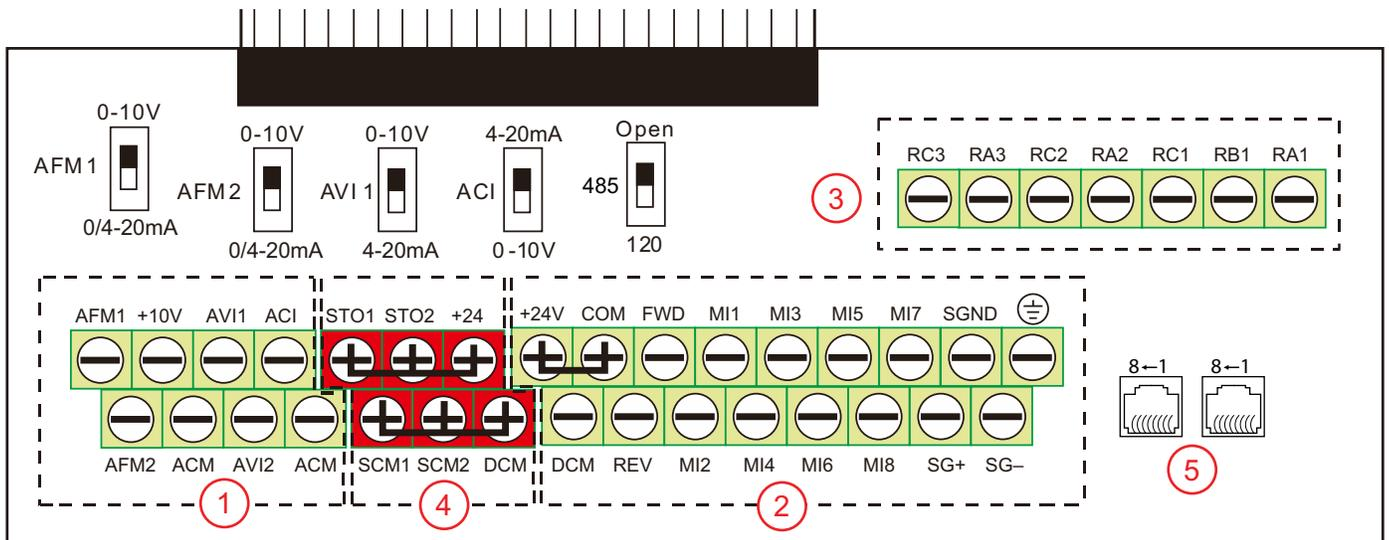
The control board is divided into 5 groups of terminals and connectors, plus a group of micro switches that control individual terminal configurations.
