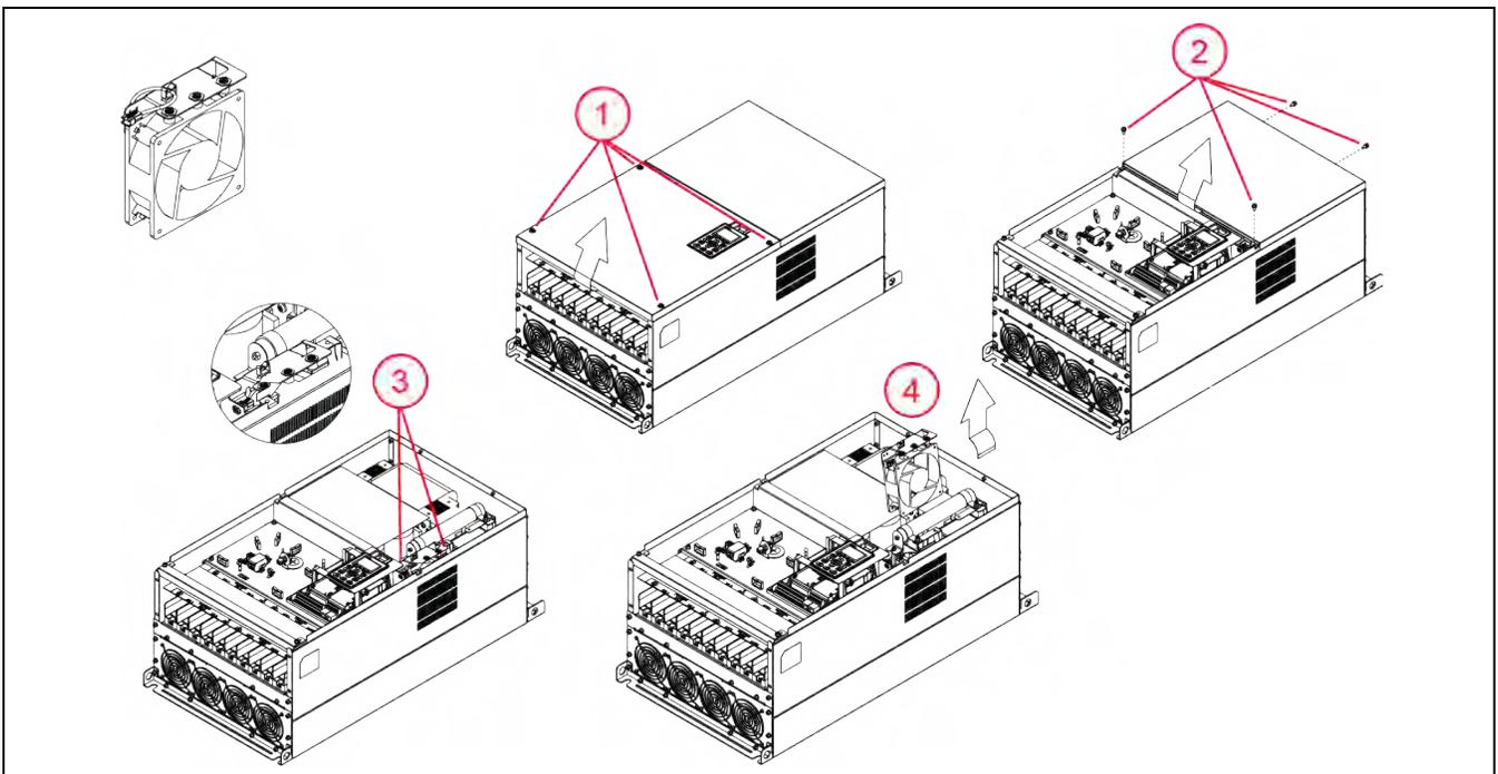
1. Remove four screws and remove the lower cover. When replacing screws, tighten to a torque of 10.4 to 13 in. lbs. (1.18 to 1.47 Nm).
