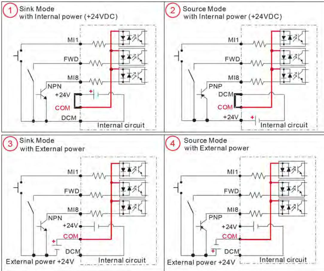
The picture above shows four possible digital inputs configurations:
