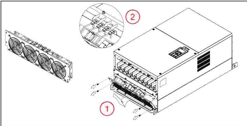
1. Remove four screws to release and slide out the fan assembly. When replacing screws, tighten to a torque of 10.4 to 13 in. lbs. (1.18 to 1.47 Nm).
