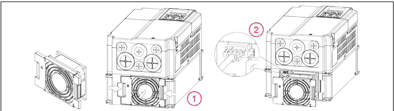
1. Press the tabs on both sides of the fan to release and slide out the fan.
