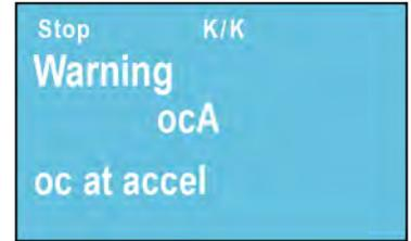
**Fault Records:** In addition, the drive records up to 30 of the most recent faults. These can be accessed by pressing the **F3** key. Use the arrow keys to scroll through the list. For more information about a selected fault, press the **Enter** key to display details about the occurrence, including date, time, output frequency, output current, and other related data.
