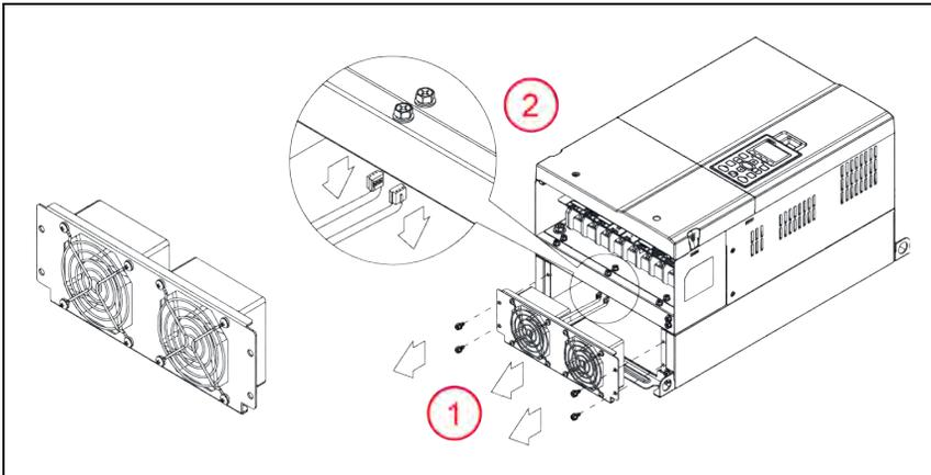
1. Remove four screws to release and slide out the fan assembly. When replacing screws, tighten to a torque of 20.8 to 22.1 in. lbs. (2.35 to 2.5 Nm).
