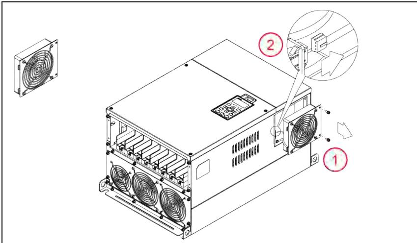
Frame E models use multiple heat sink fan styles. Be sure to order the correct part when replacing the fan.
