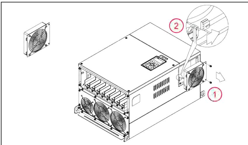
1. Remove four screws to release and slide out the fan assembly. When replacing screws, tighten to a torque of 20.8 to 22.1 in. lbs. (2.35 to 2.5 Nm).
