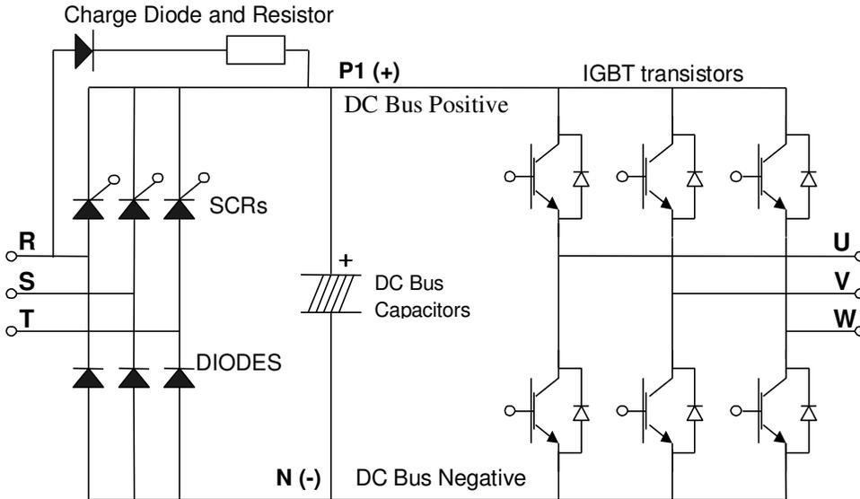
Note: The 50-700HP VFDs have half controlled rectifier bridge with SCRs (silicon controlled rectifier). The SCR cannot be checked for conducting state with multimeter. The reading from R to P1 terminals will represent charge diode and resistor circuit. Terminals S and T to P1 will show closed state in direct and reverse test if SCRs are not shorted.
