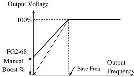
for Forward Boost and FG2-69 for Reverse Boost. The Torque Boost value is a percentage of SET-08 Motor Voltage. If FG1-40 V/F Pattern is set to User V/F, the torque boost function is disabled.
