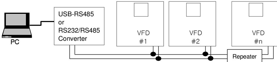
Note: The repeater is used for long-distance communication or high noise environment.
