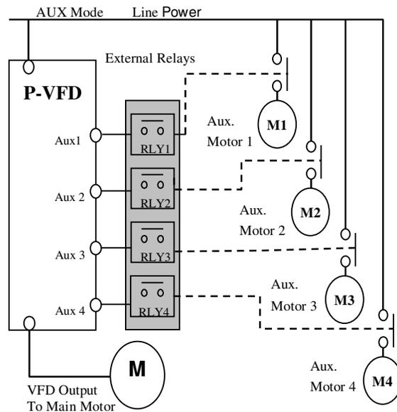
**Main-** the alternation mode is enabled and VFD will alternate auxiliary motors on the VFD output by run time timer.
