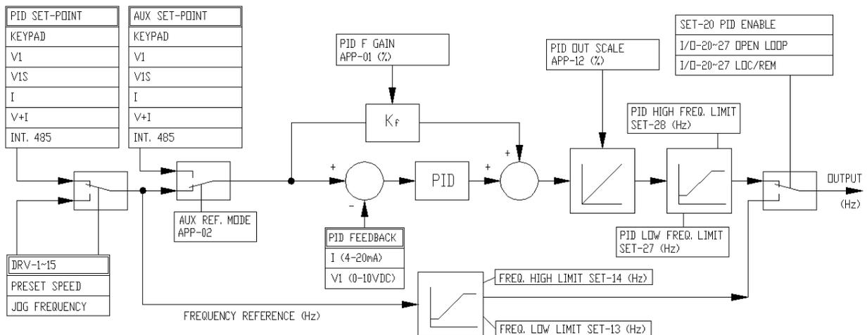
The picture above shows a PID block diagram with most of the required PID operation parameters. The PID output (Target) and VFD output frequency (Out) can be viewed on parameter DRV-25 screen.
