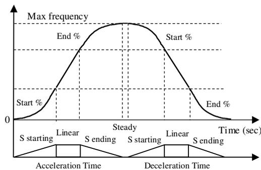
$$\text{The Actual Accel time} = [\text{SET} - 11] + \left( \frac{[\text{SET} - 11] \times [\text{FG1} - 03]}{2} \right) + \left( \frac{[\text{SET} - 11] \times [\text{FG1} - 04]}{2} \right).$$
