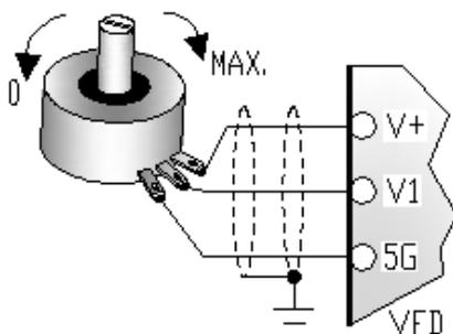
VFD speed control potentiometer wiring with VFD internal 12VDC power supply. The recommended potentiometer parameters: Resistance from 1kΩ to 10kΩ and Wattage 0.5W or higher. The multi-turn potentiometer provides more precise speed adjustment compare to a single-turn potentiometer. The internal power supply provides 12VDC and in order to have full range of speed control by potentiometer, change the I/O-04 parameter from 10VDC to 12VDC.
