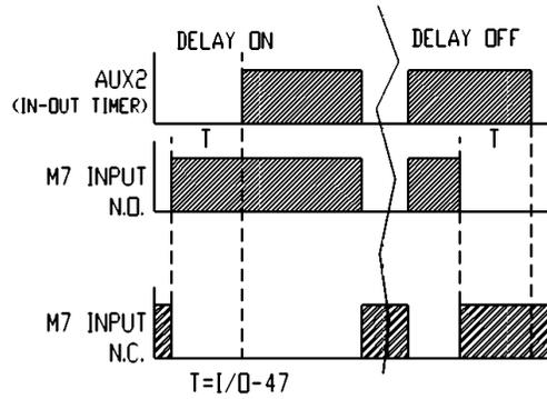
The following diagram shows timer operation in ONE Pulse and SYMM. Pulse modes with M7 as N.O. and N.C. contact and AUX2 relay set as a timer relay.
