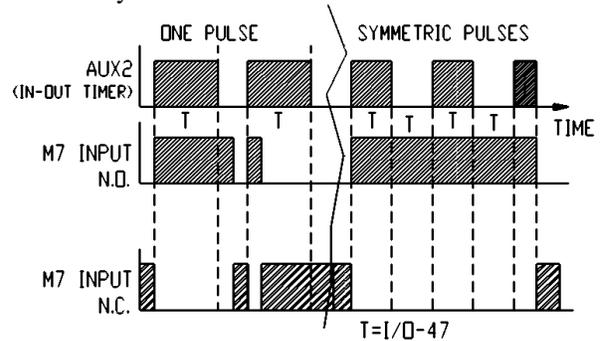
The timer set to ONE Pulse mode will generate one pulse for duration set in I/O-47 after input was activated momentarily or continuously.
