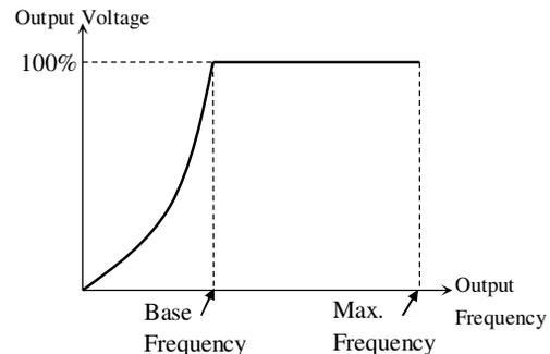
**User V/F** pattern is used for special applications with up to five different Volts/Frequency ratio step requirements. The User V/F curve can have one or two standard V/F segments and up to three custom V/F ratio segments. The parameters FG1-41~48 define Voltage and Frequency for each point on the User V/F curve.
