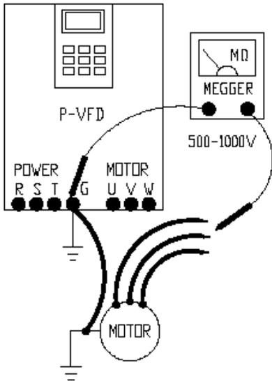
The windings insulation resistance should be in the Mega Ohm range.
