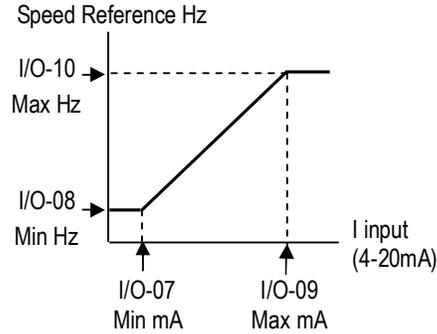
**V1+I mode.** VFD speed is controlled by both 0-10VDC and 4-20mA analog input signals from BMS, PLC, potentiometer or other control device. Both analog signals are compared with each other and the greatest value determines the VFD speed reference. The VFD speed reference can be switched between V1 and I inputs by digital input set to ANA\_CHG (Analog change). The input ranges are adjustable in I/O group parameters.
