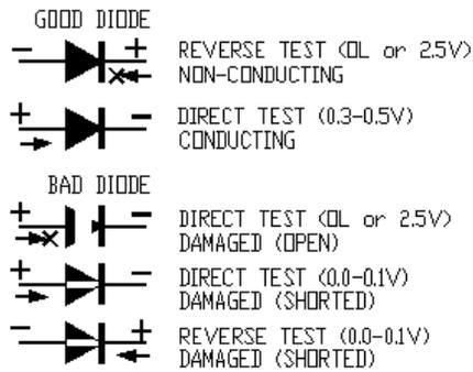
The VFD input and output power components are semiconductors and can be checked by multimeter with diode check mode (▶). When DC voltage positive is applied to the diode anode (triangle ▶) and negative to cathode (bar ▮), the diode is conducting.
