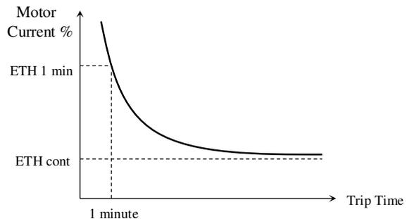
**FG1-62** sets the service factor current (SFA) as a percentage of the motor FLA for continuous run.
