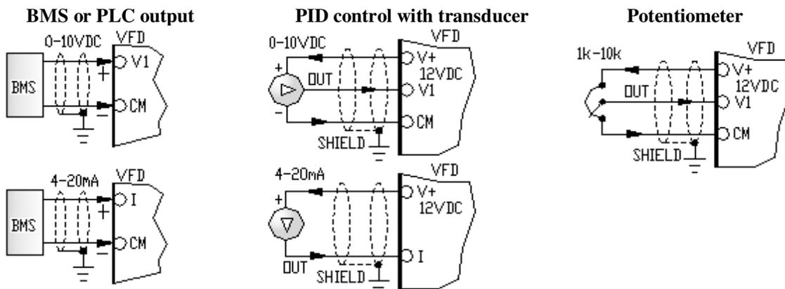
Note: See section 4.4 for more details on analog inputs wiring.
