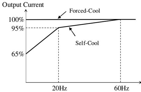
**FG1-64 & 65: VFD Overload Warning Settings**
