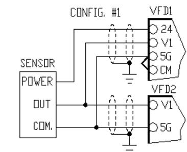
0-10VDC TRANSDUCER TO TWO VFDs WITH 24V VFD1 POWER SUPPLY
