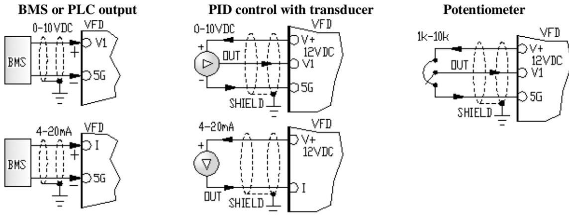
Note: See section 4.4 for more details on analog inputs wiring.
