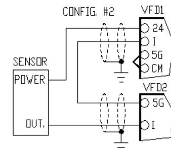
4-20mA TRANSDUCER TO TWO VFDs WITH 24V VFD1 POWER SUPPLY
