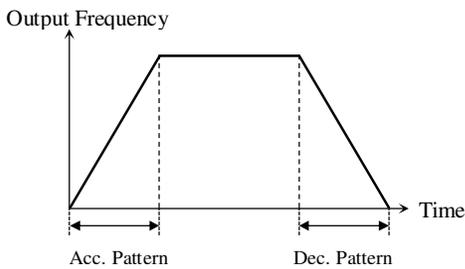
The **S-Curve** provides non-linear relation between VFD output frequency and time. The maximum and minimum frequency limits are set in SET-13 and SET-14. This pattern allows the motor to accelerate and decelerate smoothly. The actual acceleration and deceleration time will be about 40% longer than the time set in SET-11 and SET-12. The S-Curve prevents mechanical shock of the equipment during acceleration and deceleration modes.
