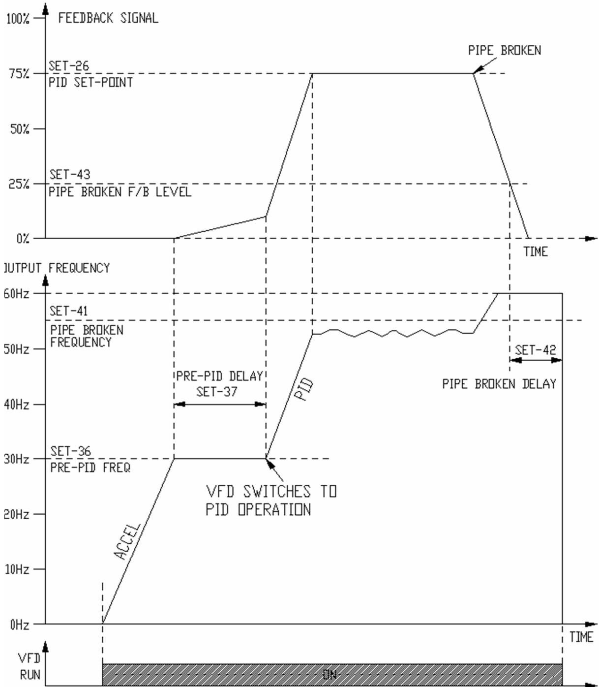
7.5 Pre-PID (Pipe Fill) function diagram.
