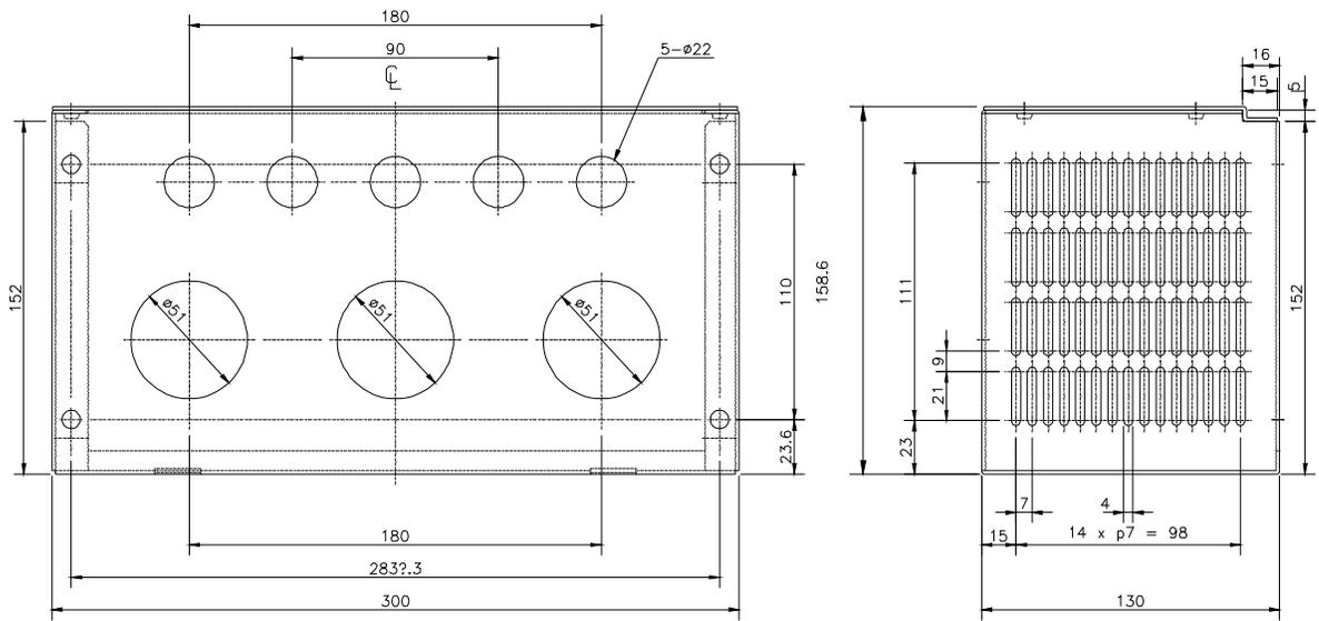
Conduit box for 050~075HP VFD
