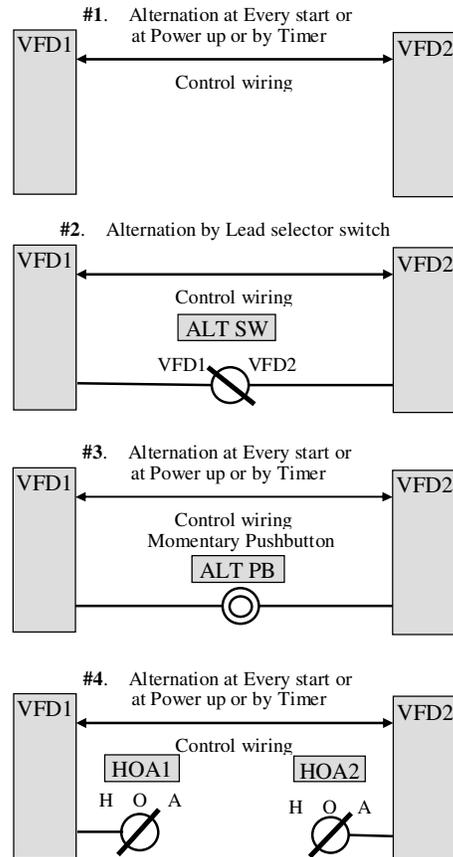
**The configuration #1** is for two VFDs with only control wiring between them. The alternation mode can be set to By Timer , At Power up or can be configured for alternation at Every start.
