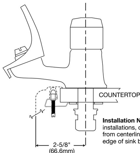
**Installation Note:** For countertop installations, do not exceed 2-5/8" from centerline of bubbler hole to edge of sink bowl as shown.
