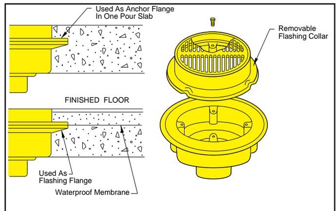
Most floor drain bodies are available with a flange for either anchoring the drain in the floor slab or for use as a flashing flange in upper floors and waterproofed areas. Many Smith drains are regularly furnished with a flanged body and a combination "top flashing collar" which can be used to clamp the waterproof membrane.
