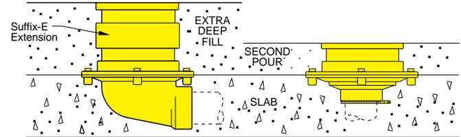
Adjustable drains are particularly useful in areas where the finished floor elevation may vary or is not immediately determined. Additional adjustable extension sleeve is available for extra deep roughing conditions (Specify Suffix -E).
