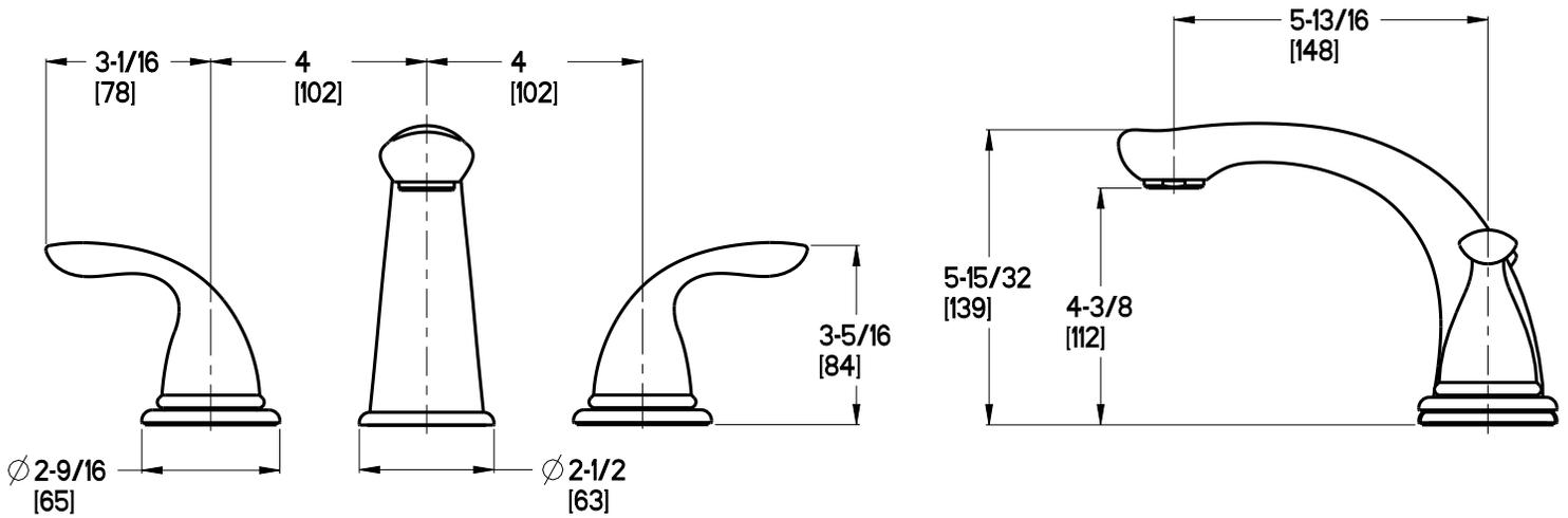
$\phi$ 1 Min to  $\phi$ 1-1/2 Max. Deck Hole Openings
