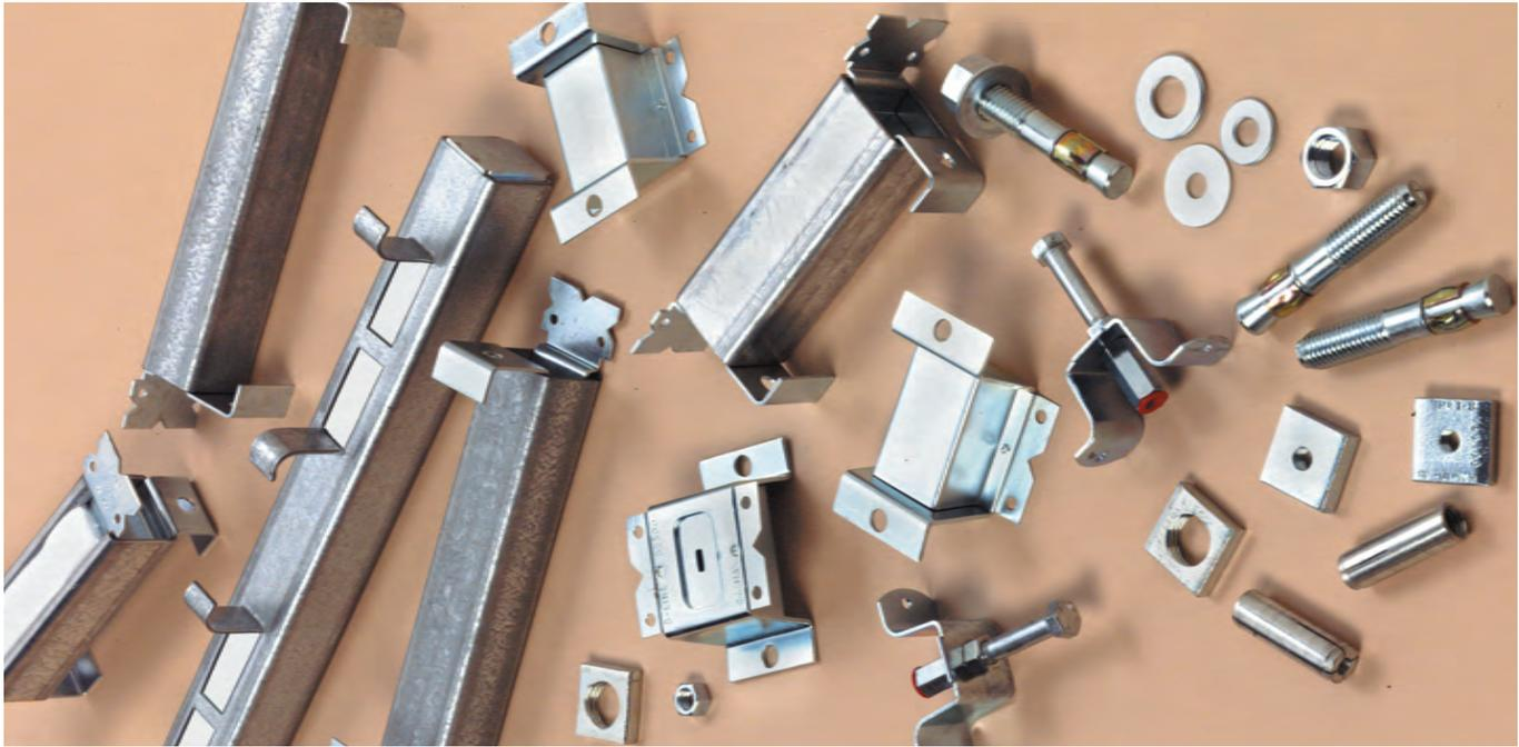
Continuous slot concrete inserts are designed to provide a pre-set support system cast in concrete ceilings, walls, and floors to allow flexibility of attachment at any point along the channel. This provides an excellent support system for pipe, conduit, and cable trays.
