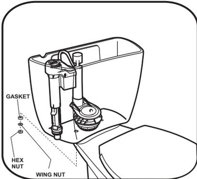
**5** ONCE THE TANK IS PLACED ON THE BOWL, INSERT GASKET AND WASHER ON THE SCREW; ONCE INSERTED, TIGHTEN HEX NUT UNTIL TANK IS WELL SECURED; BE SURE NOT TO OVERTIGHTEN FOR IT COULD BREAK THE TANK.
