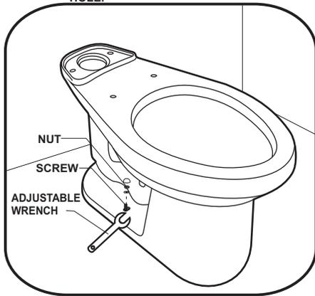
**2** REMOVE TOILET SEAT FROM ITS BOX AND PLACE IT IN NORMAL POSITION ON THE TOILET FLANGE, WITH THE SCREWS INSIDE ITS BASE; BE SURE IT STANDS STRAIGHT. NEXT, PLACE THE NUTS AND SECURE THEM WELL WITH AN ADJUSTABLE WRENCH.
