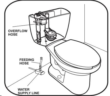
**7** TO SUPPLY WATER TO THE TOILET USE A FEEDING HOSE, WHICH HAS TO BE CONNECTED TO THE WATER SUPPLY LINE.
