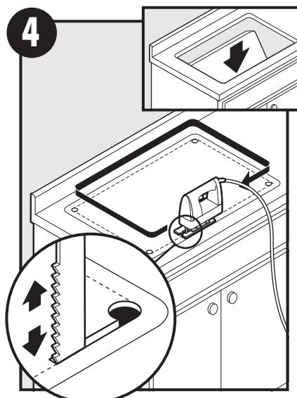
Carefully cut counter hole following inside of the cut line. Remove counter material.
