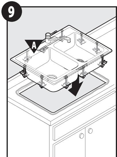
Center sink within counter opening. Apply even pressure to all sides. Wipe away any excess caulk on counter.
