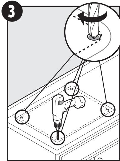
Drill pilot holes on cut line.
