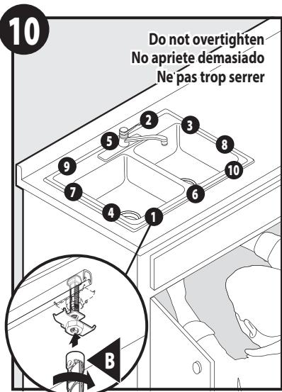
Tighten installation screws with mounting tool in order as shown above.
