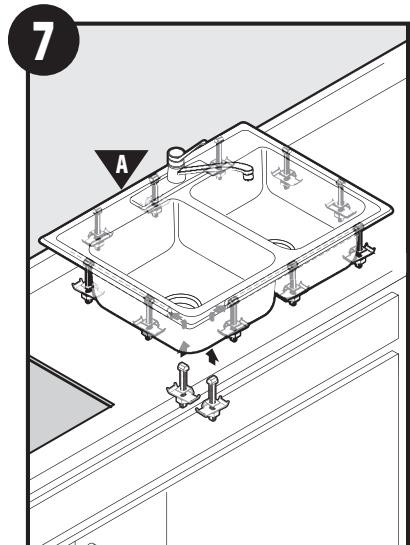
Insert mounting hardware onto sink mounting rails along each side as illustrated. 10 total mounting hardware included.
