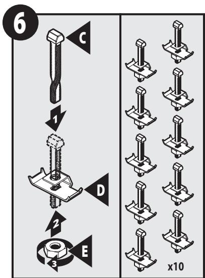
Insert clip onto screw and thread on nut maximum of 2 turns.
