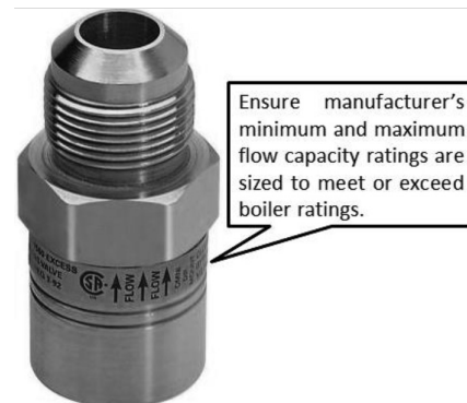
Figure 29 - Excess Flow Valve (EFV)
