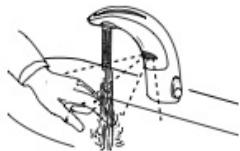
As the user's hands enter the beam's effective range, the beam is reflected back into the sensor receiver and activates the solenoid valve allowing water to flow from the faucet. Water will flow until the hands are removed or until the faucet reaches its automatic time out limit setting.
