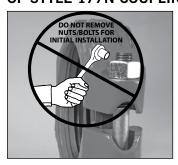
1. DO NOT DISASSEMBLE THE COUPLING: Style 177N QuickVic™ Installation-Ready™ Flexible Couplings are designed so that the installer does not need to remove the bolts and nuts for installation. This design facilitates installation by allowing the installer to directly insert the grooved end of mating components into the coupling.
