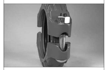
METHOD 1 FOR RE-INSTALLATION: The coupling can be re-assembled into its "installation-ready" condition by installing the gasket into the housings, then inserting the bolts and threading a nut onto each bolt until 2 – 3 threads are exposed, as shown above. If this method is chosen, steps 1 – 3 above, along with steps 5 – 7 on pages 1 and 2, must be followed.
