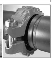
**5. ASSEMBLE JOINT:** Assemble the joint by inserting the grooved end of a mating component into each opening of the coupling. The ends of the grooved mating components must be inserted into the coupling until contact with the center leg of the gasket occurs. A visual check is required to ensure the coupling keys align with the grooves in the mating components. **NOTE:** The coupling may be rotated to ensure the gasket is seated properly.
