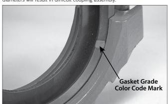
**3. CHECK GASKET:** Check the gasket to make sure it is suitable for the intended service. The color code identifies the gasket grade. Refer to Victaulic publication 05.01 in the G-100 General Catalog for the color code chart.
