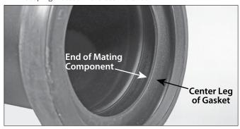
**2. INSTALL GASKET:** Insert the grooved end of a mating component into the gasket until it contacts the center leg of the gasket.
