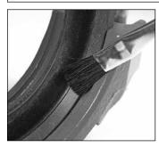
4. LUBRICATE GASKET: Apply a thin coat of Victaulic Lubricant or silicone lubricant only to the sealing lips of the gasket interior. NOTE: The gasket exterior is supplied with a factory-applied lubricant, so it is not necessary to remove the gasket from the housings to apply additional lubricant to the exterior surface.
