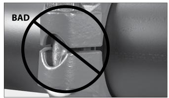
7. Visually inspect the bolt pads at each joint to ensure metal-to-metal contact is achieved across the entire bolt pad section.
