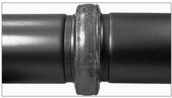
**3. JOIN MATING COMPONENTS:** Align the two grooved ends of the mating components. Insert the other mating component end into the gasket until it contacts the center leg of the gasket. **NOTE:** Make sure no portion of the gasket extends into the groove of either mating component.
