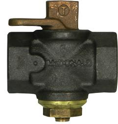
Cast iron body, brass plug manually operated 175 PSIG natural, manufactured, or propane gas valve for use in above ground gas piping systems in ambient temperatures between -20°F to 150°F. Iron body valves considered full port of flow. Made in the USA.
