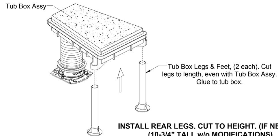
**INSTALL REAR LEGS. CUT TO HEIGHT. (IF NEEDED)
