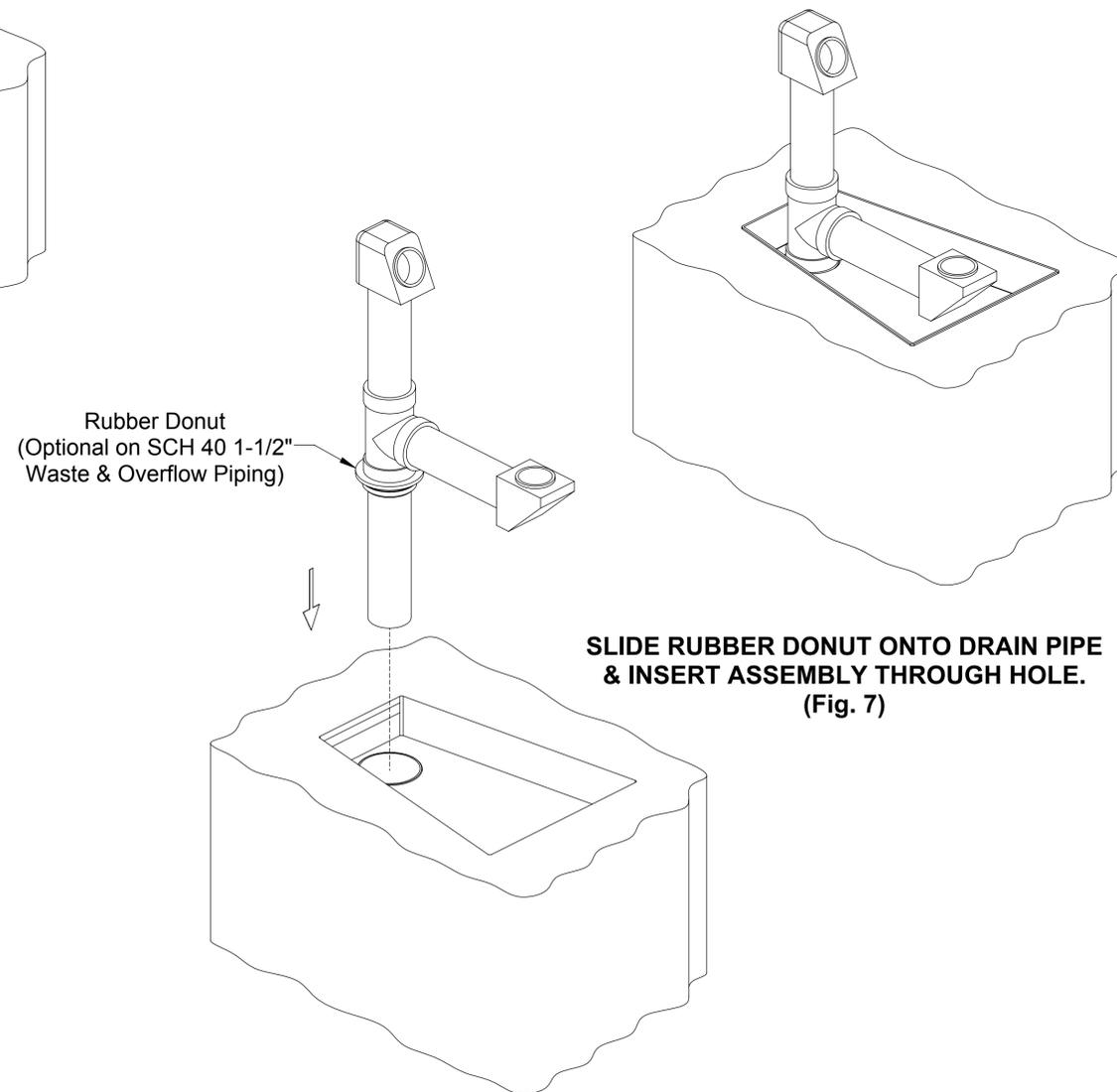
**SLIDE RUBBER DONUT ONTO DRAIN PIPE
