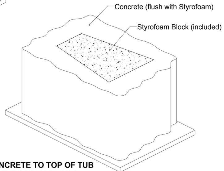
**POUR CONCRETE TO TOP OF TUB
