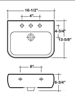
Dimensions of fixture are nominal and may vary within the range of tolerances established by ASME Standard A112.19.2.2013 Dimensions and specifications subject to change without notice.
