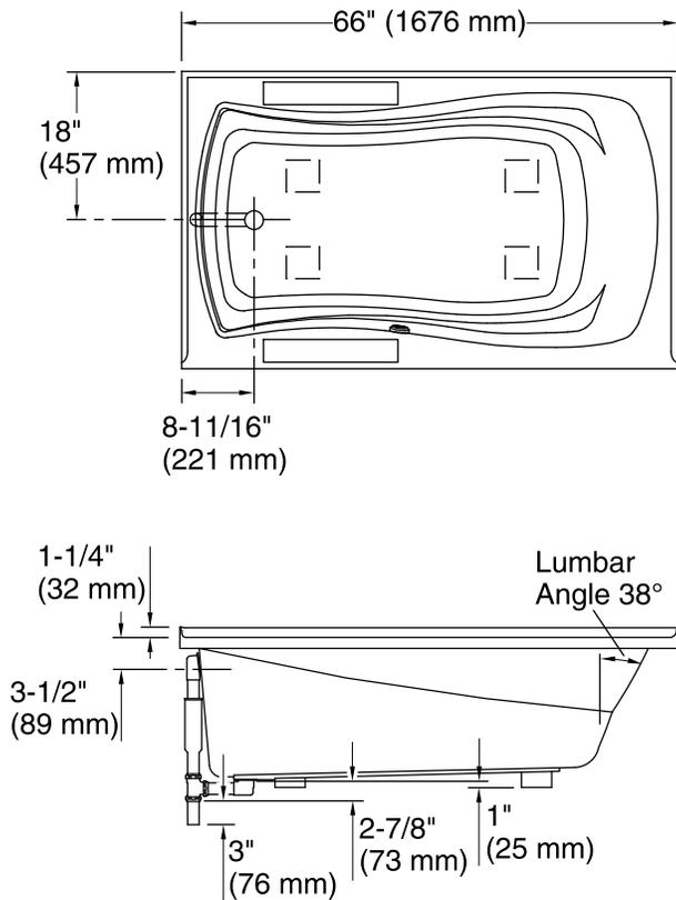
No change in measurements if connected with drain illustrated. (K-7161-AF)
