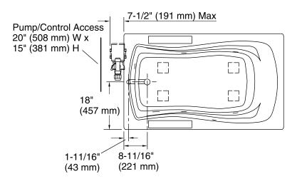
No change in measurements if connected with drain illustrated. (K-7161-AF)
