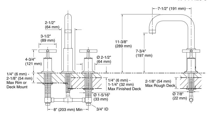
Rim or Deck-Mount Installation Rough + Finished Deck-Mount Installation
