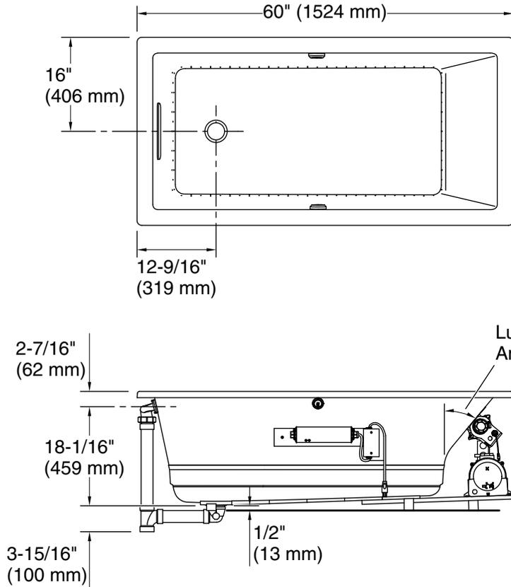
No change in measurements if connected with drain illustrated. (K-7272)
