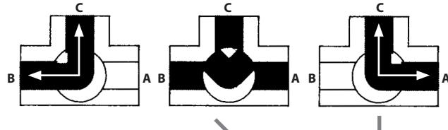
NOTE: Open port pressure must exceed Closed port pressure.
