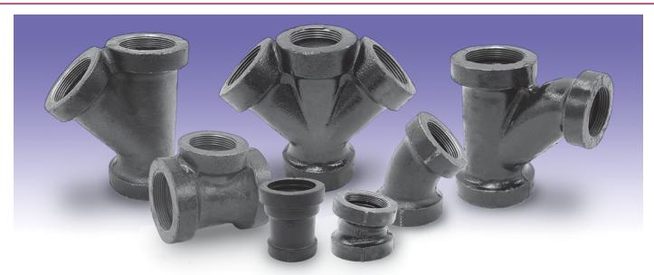
Anvil drainage fittings have sufficient sweep to allow free unobstructed flow. They are made with a shoulder of the same diameter as the inside of the pipe, in accordance with ASME B16.12, Type 1. Thus, continuous passage is created when the pipe is screwed to the shoulder, leaving no place for solid matter to collect and clog in the pipe.
