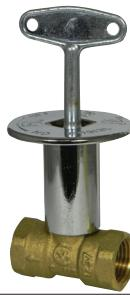
Straight and angle log lighter valves are constructed of heavy-duty forged brass with chrome or polished brass escutcheon. They have a teflon seat and a viton rubber synthetic fiber stem seal. The extremely high B.T.U. capacity makes them a good choice for either natural or artificial fireplaces. Valves are designed for use with natural, manufactured or LP gas only.
