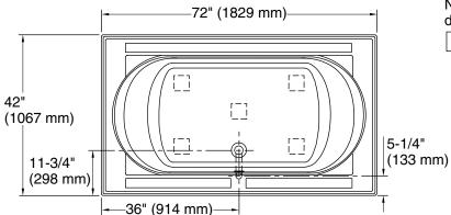
No change in measurements if connected with drain illustrated. (K-7161-AF)
