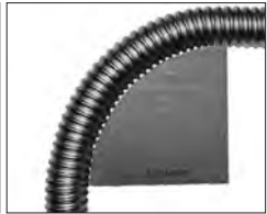
4-INCH/102-MM MINIMUM BEND RADIUS
