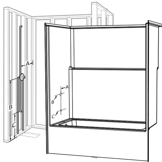
3. Mark fitting locations. (Refer to measurements from step 2.) Using a hole saw (fine tooth or abrasive grit cutting edge), make necessary openings for filler and valves, drilling from inside (smooth side) out. See Figures 3A and 3B.
