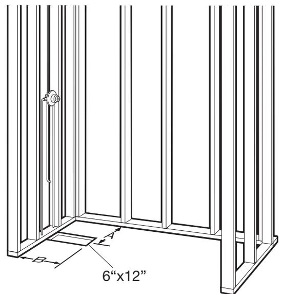
2. If mounting fittings — from stable reference points (back wall studs, floor) measure the locations of spout and valves. Note measurements below. See Figures 2A and 2B.
