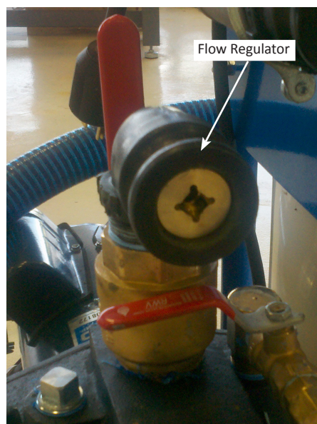
Figure 1: Flow regulator installed in 1-1/2" cam supply
