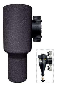
Manufactured from Expanded Polypropylene (EPP) the Fernox TF1 Total Filter Thermal Cover is used to insulate inline system filters installed on central heating systems to minimise system heat loss and maximise energy efficiency
